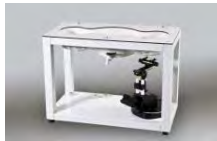
Figure E.5.1 SAM Twin Phantom
