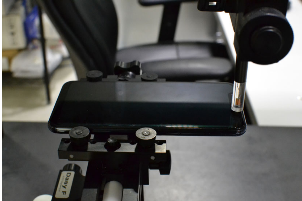
Figure 16-1 Test Setup for Wireless Device
