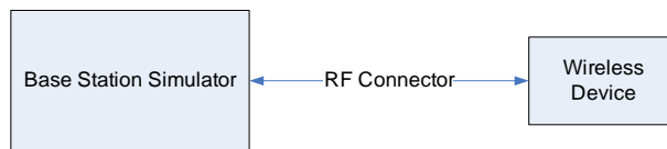
Figure 9-2 Power Measurement Setup
