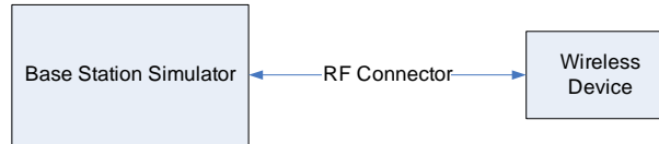
Figure 9-4 Power Measurement Setup
