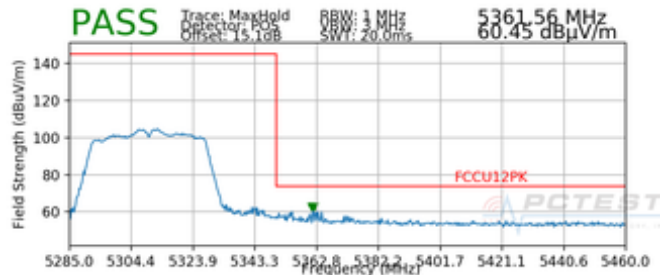
Plot 7-55. Radiated Upper Band Edge Plot SISO ANT2 (Peak – UNII Band 2A)
