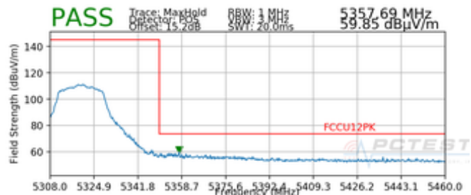
Plot 7-46. Radiated Upper Band Edge Plot SISO ANT2 (Peak – UNII Band 2A)
