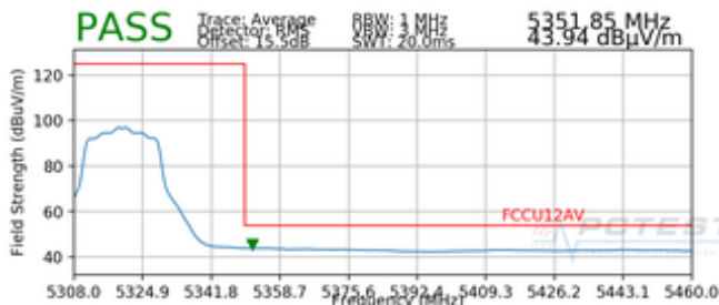
Plot 7-18. Radiated Upper Band Edge Plot SISO ANT1 (Average – UNII Band 2A)
