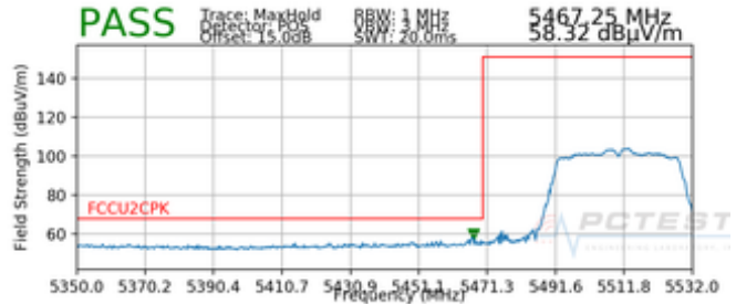
Plot 7-57. Radiated Lower Band Edge Plot SISO ANT2 (Peak – UNII Band 2C)
