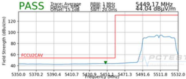
Plot 7-56. Radiated Lower Band Edge Plot SISO ANT2 (Average – UNII Band 2C)
