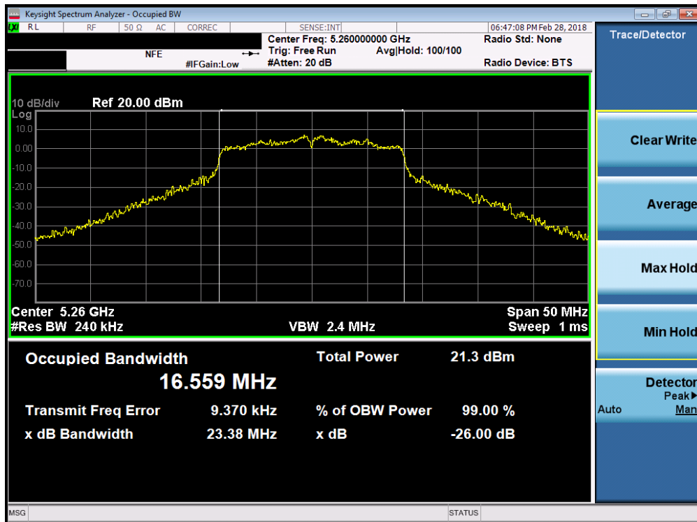
Plot 7-40. 26dB Bandwidth Plot (802.11a (UNII Band 2A) – Ch. 52)
