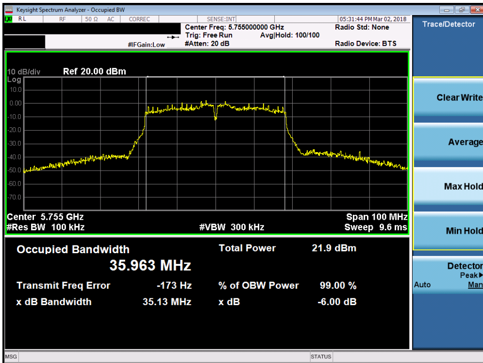
Plot 7-67. 6dB Bandwidth Plot (40MHz BW 802.11n (UNII Band 3) – Ch. 151)
