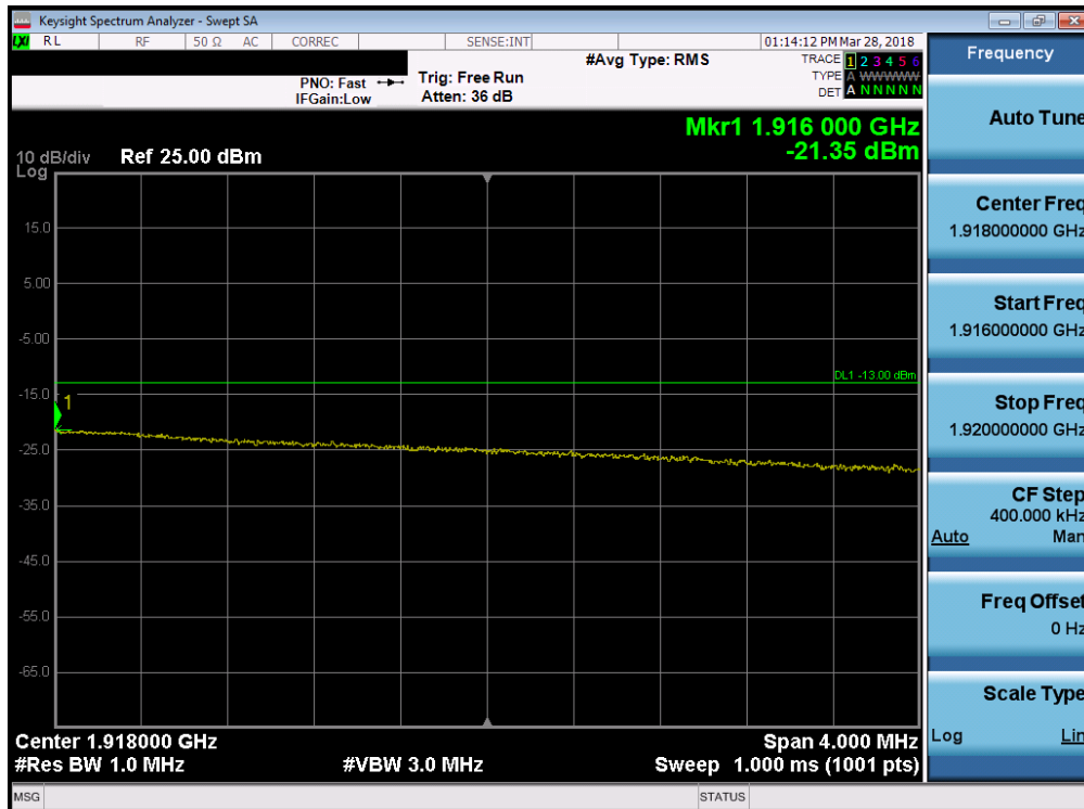
Plot 7-228. Extended Upper Band Edge Plot (Band 25 - 20.0MHz QPSK - Full RB Configuration)
