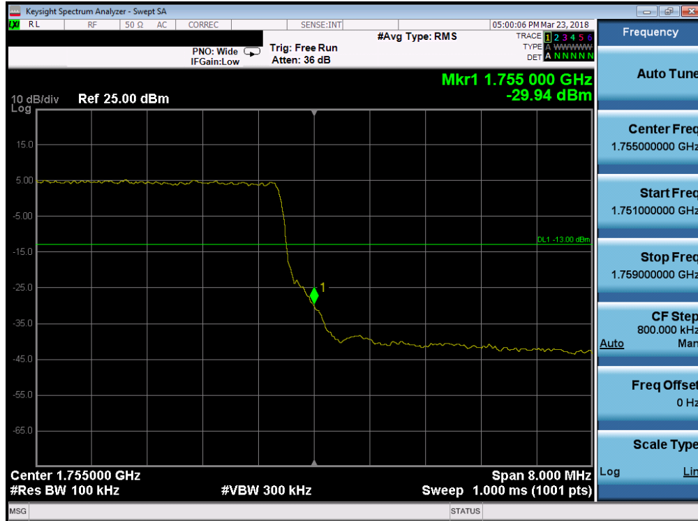
Plot 7-177. Upper Band Edge Plot (Band 4 - 10.0MHz QPSK - Full RB Configuration)
