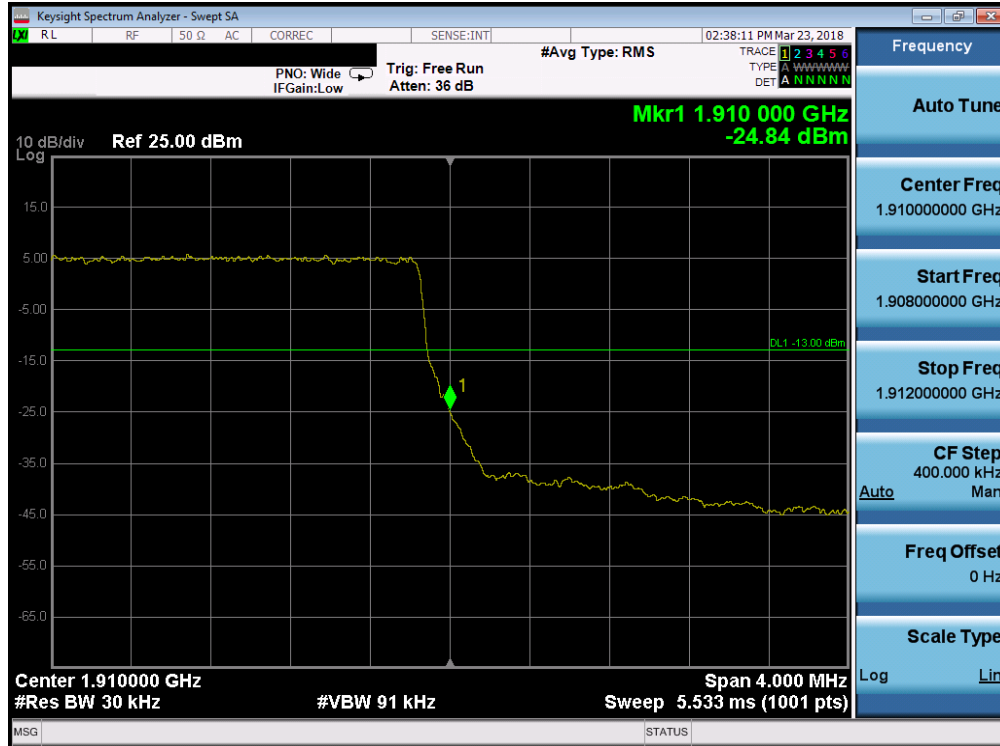
Plot 7-201. Upper Band Edge Plot (Band 2 - 3.0MHz QPSK - Full RB Configuration)
