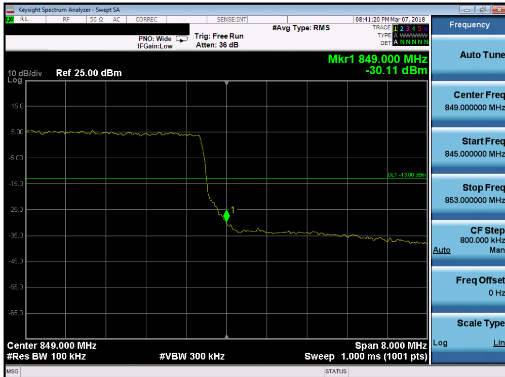
Plot 7-154. Upper Band Edge Plot (Band 26/5 - 10.0MHz QPSK - Full RB Configuration)
