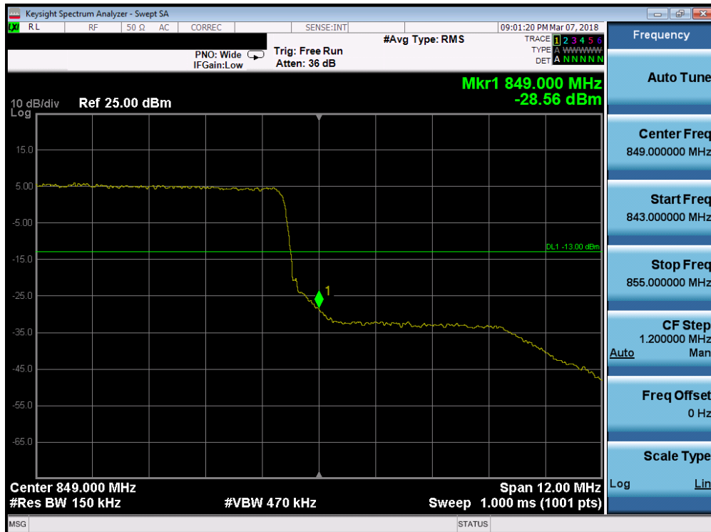
Plot 7-156. Upper Band Edge Plot (Band 26 - 15.0MHz QPSK - Full RB Configuration)
