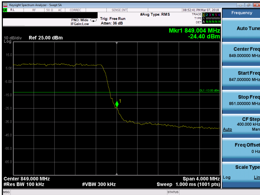
Plot 7-152. Upper Band Edge Plot (Band 26/5 - 5.0MHz QPSK - Full RB Configuration)
