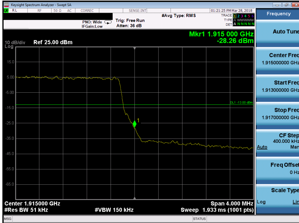
Plot 7-209. Upper Band Edge Plot (Band 25 - 5.0MHz QPSK - Full RB Configuration)
