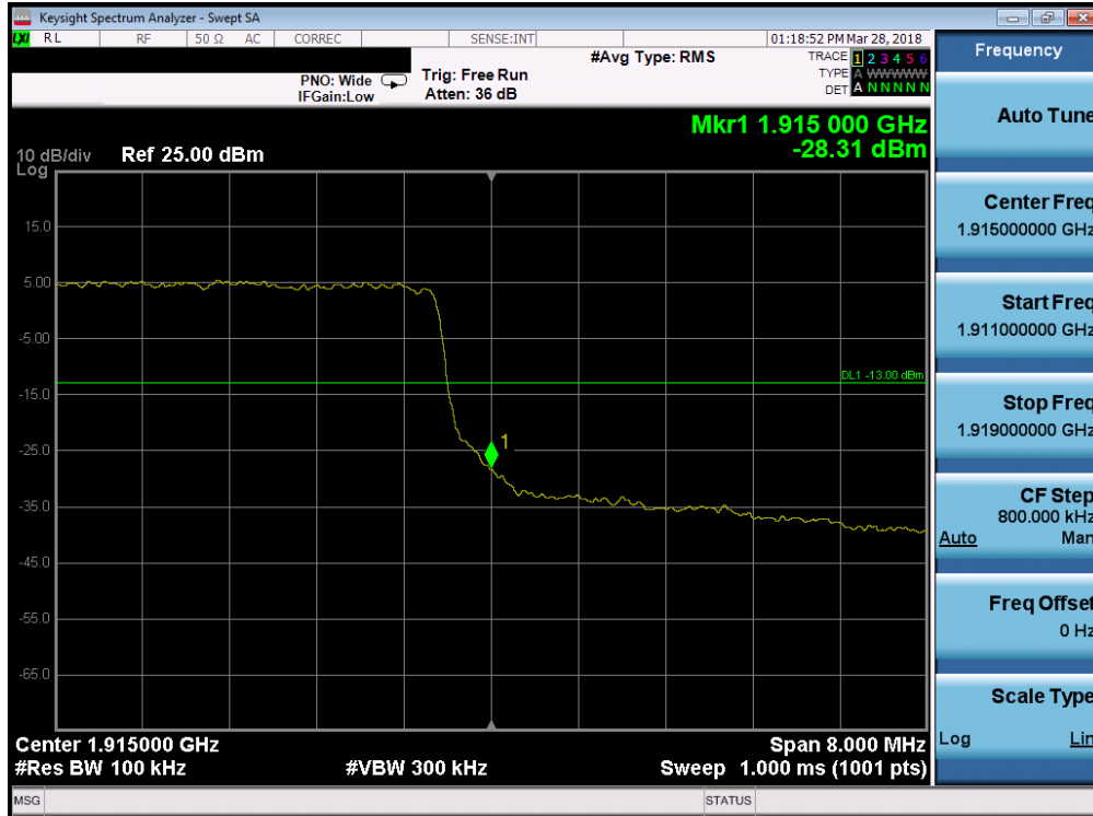
Plot 7-215. Upper Band Edge Plot (Band 25 - 10.0MHz QPSK - Full RB Configuration)
