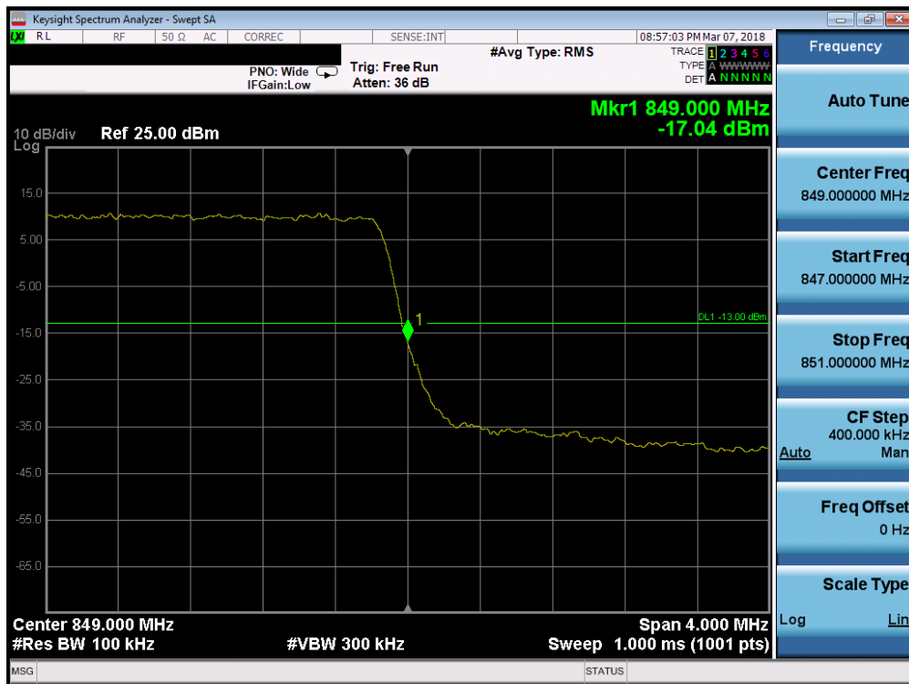
Plot 7-150. Upper Band Edge Plot (Band 26/5 - 3.0MHz QPSK - Full RB Configuration)
