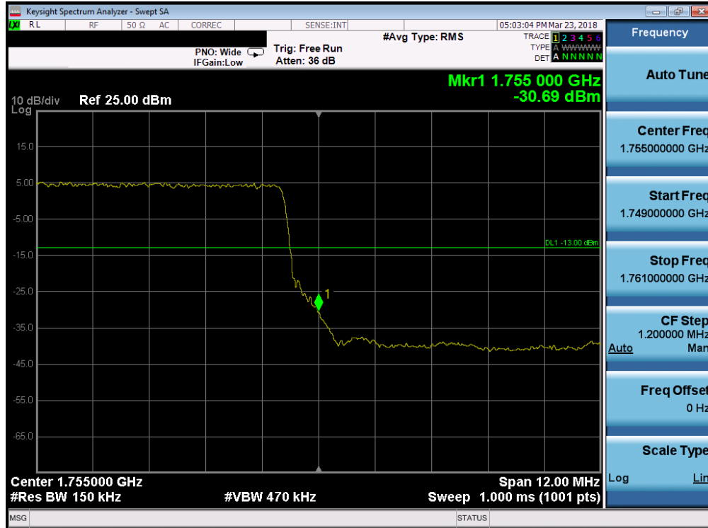
Plot 7-183. Upper Band Edge Plot (Band 4 - 15.0MHz QPSK - Full RB Configuration)
