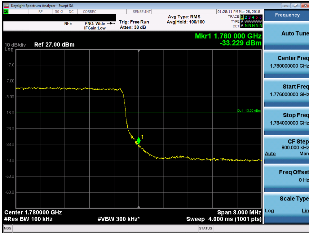
Plot 7-179. Upper Band Edge Plot (Band 66 - 10.0MHz QPSK - Full RB Configuration)
