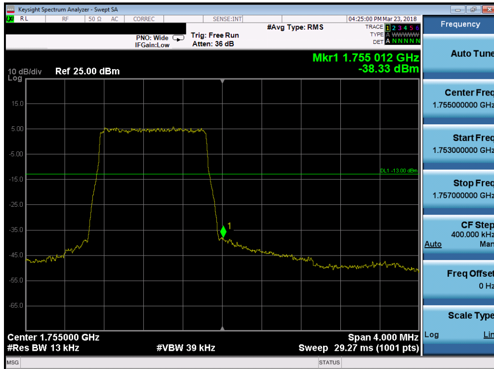
Plot 7-159. Upper Band Edge Plot (Band 4 - 1.4MHz QPSK - Full RB Configuration)
