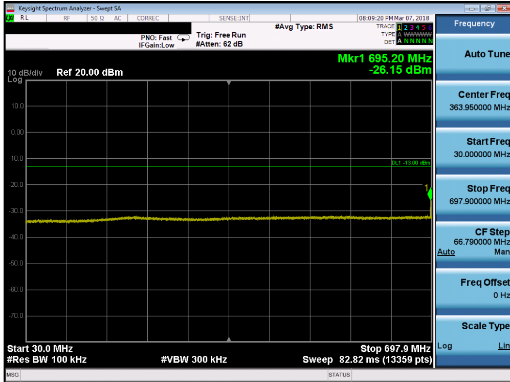
Plot 7-82. Conducted Spurious Plot (Band 12/17 - 10.0MHz QPSK - RB Size 1, RB Offset 0 - Low Channel)
