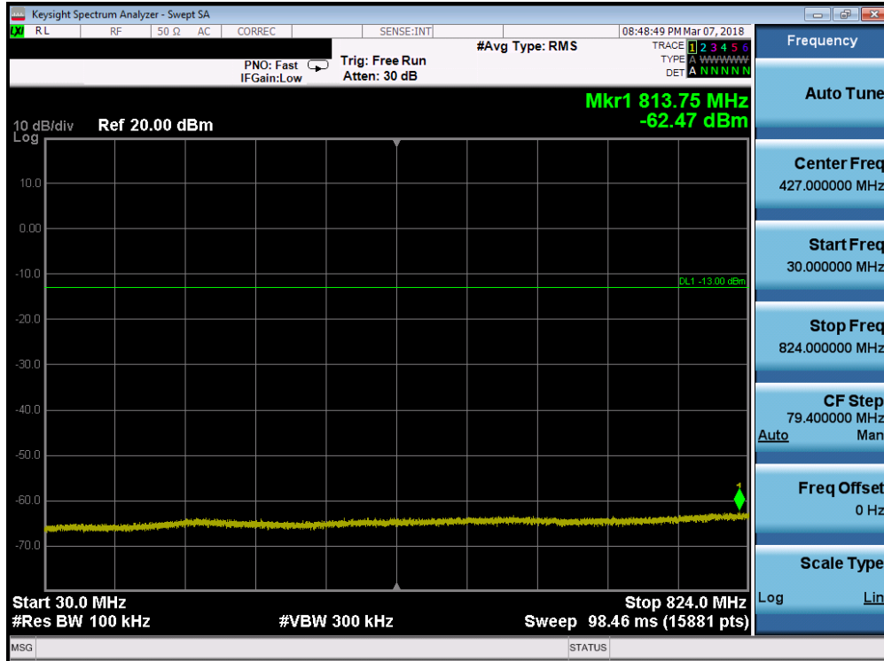
Plot 7-103. Conducted Spurious Plot (Band 26/5 - 5.0MHz QPSK - RB Size 1, RB Offset 0 - High Channel)
