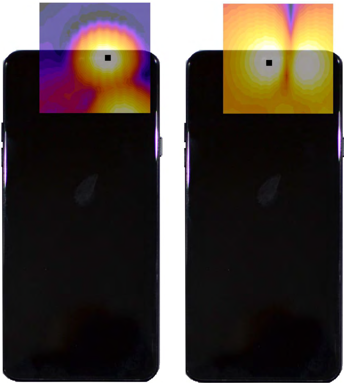
Figure 16-3 T-Coil Scan Overlay Magnetic Field Distributions
