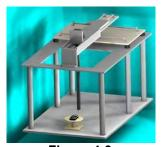
Figure 4-3 RF Near-Field Scanner
