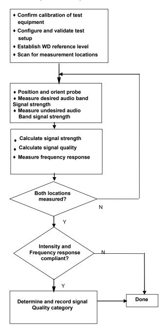
Figure 4-15 C63.19 T-Coil Signal Test Process
