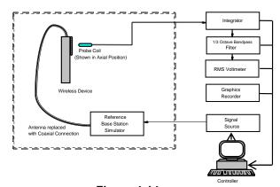
Figure 4-14 **Audio Magnetic Field Test Setup**
