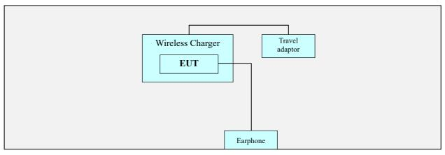
**Non-Conductive Table** Power Line: 120 VAC, 60 Hz
