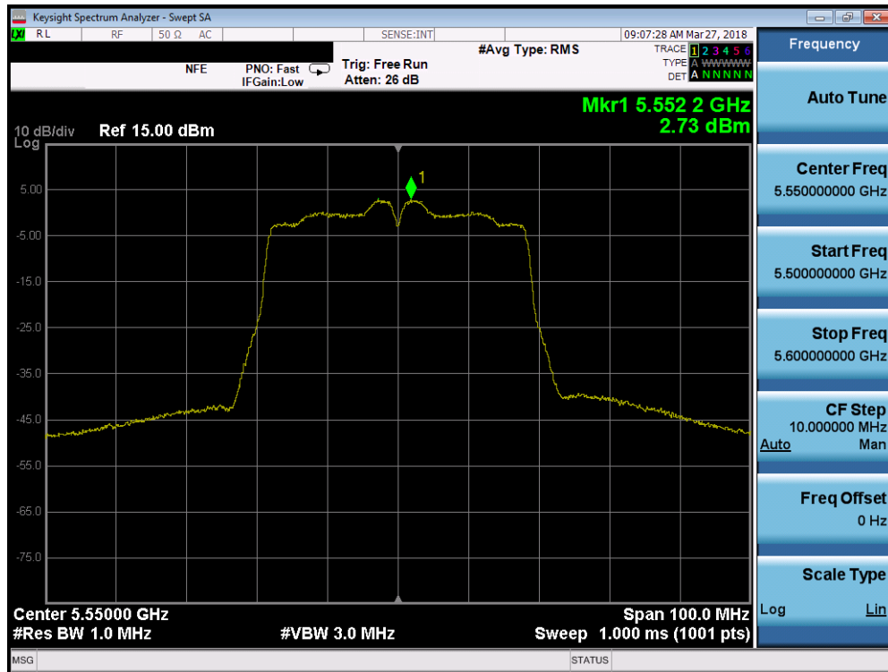
Plot 7-102. Power Spectral Density Plot (40MHz BW 802.11n (UNII Band 2C) – Ch. 110)
