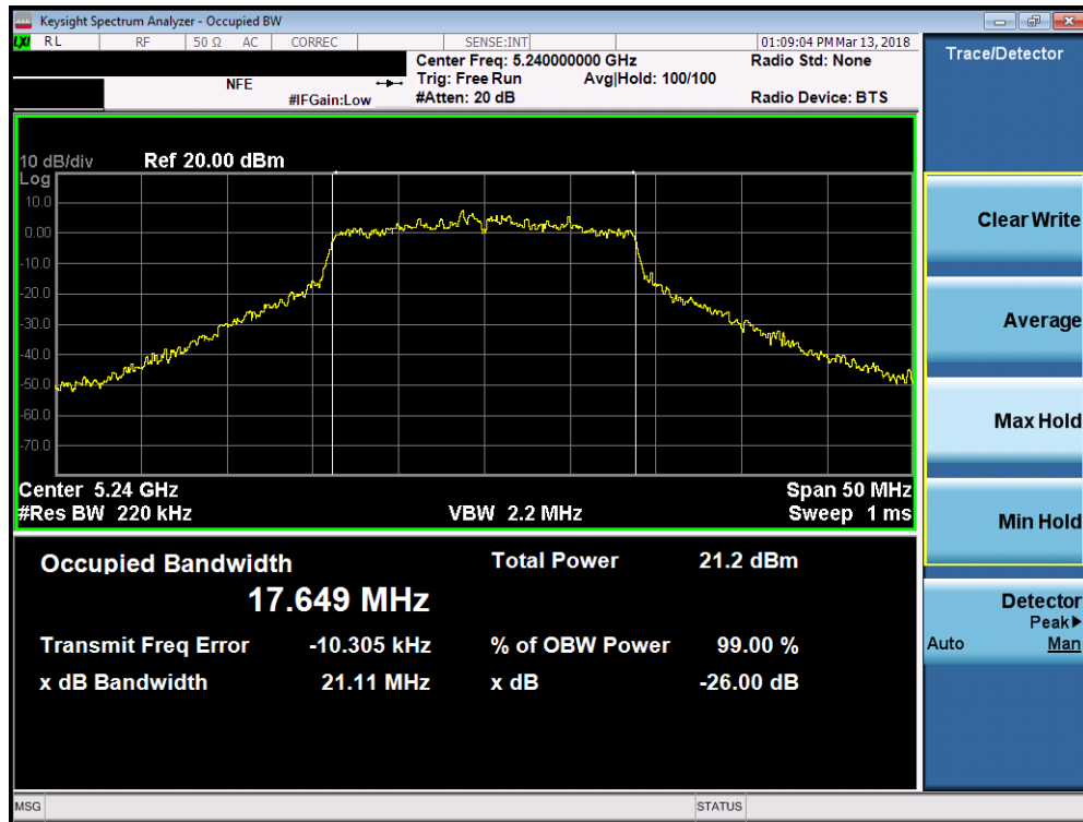
Plot 7-35. 26dB Bandwidth Plot (20MHz BW 802.11n (UNII Band 1) – Ch. 48)
