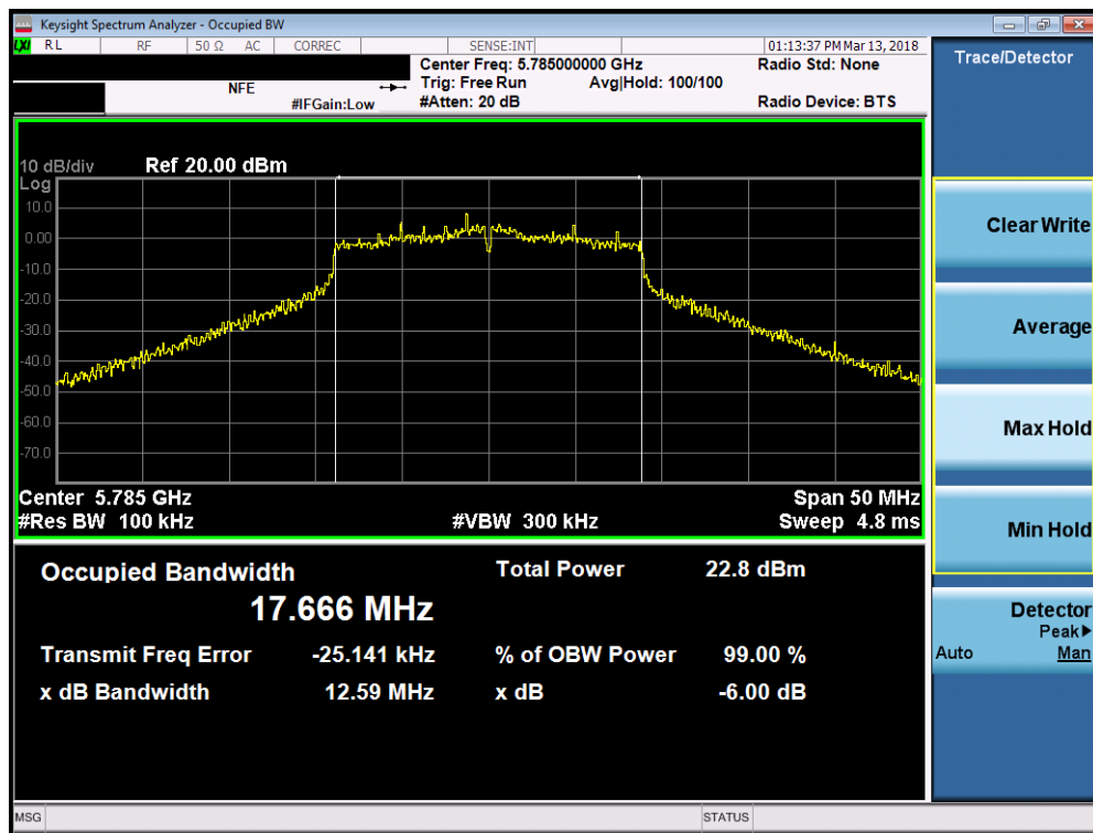
Plot 7-72. 6dB Bandwidth Plot (20MHz BW 802.11n (UNII Band 3) – Ch. 157)
