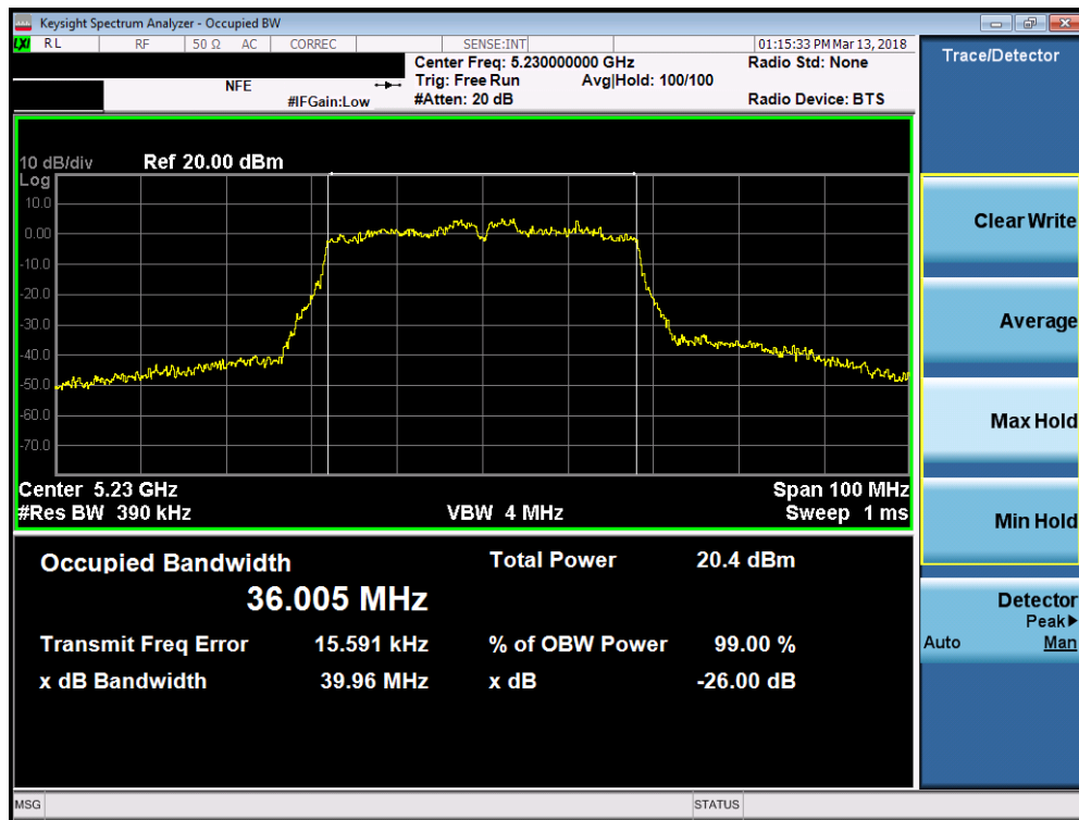
Plot 7-37. 26dB Bandwidth Plot (40MHz BW 802.11n (UNII Band 1) – Ch. 46)
