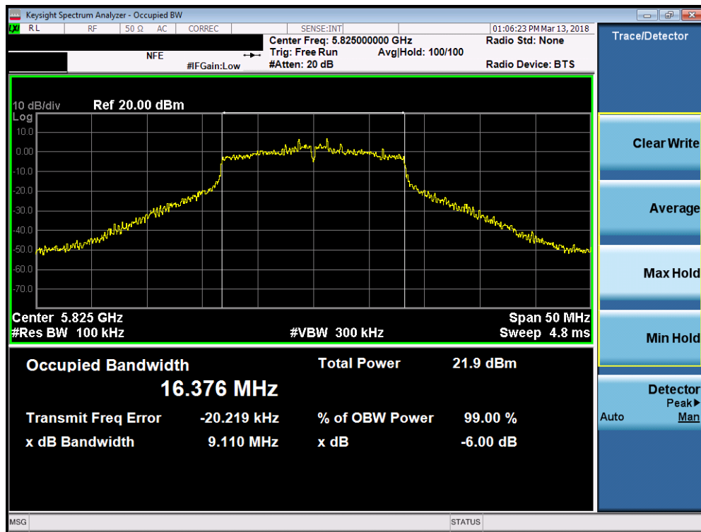
Plot 7-70. 6dB Bandwidth Plot (802.11a (UNII Band 3) – Ch. 165)
