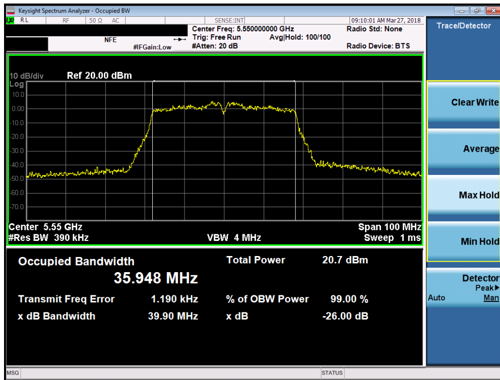
Plot 7-55. 26dB Bandwidth Plot (40MHz BW 802.11n (UNII Band 2C) – Ch. 118)
