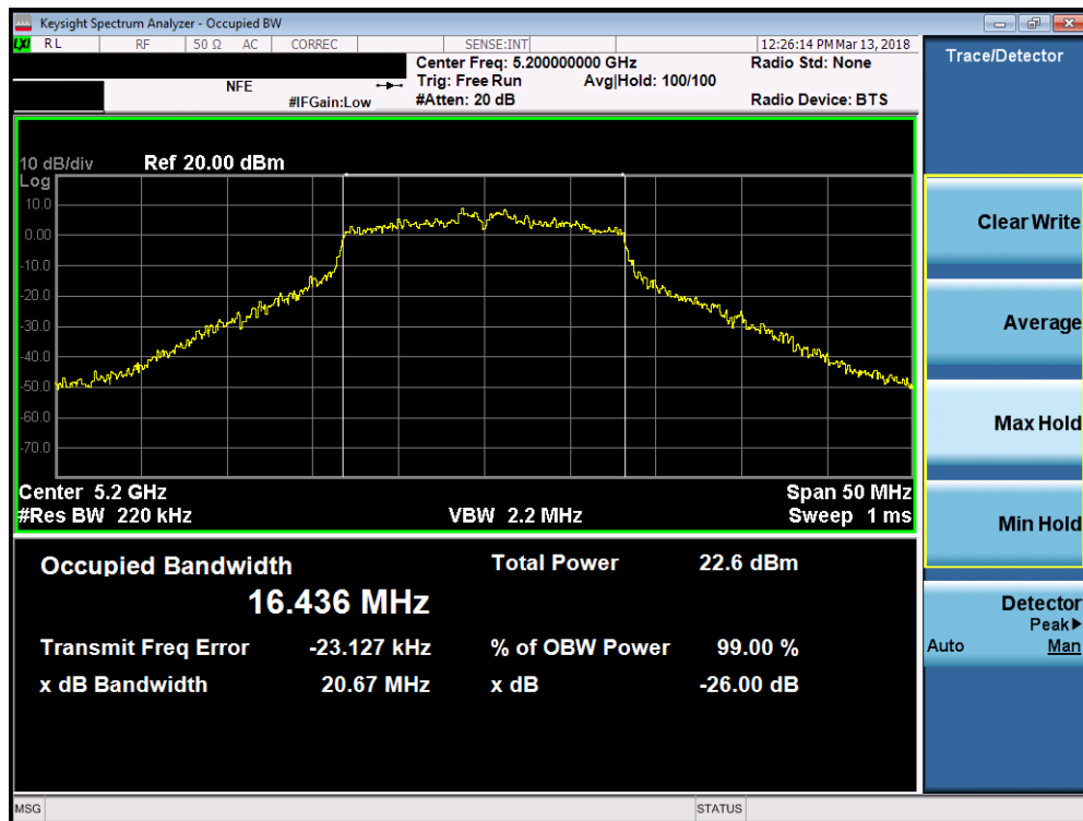
Plot 7-2. 26dB Bandwidth Plot (802.11a (UNII Band 1) – Ch. 40)
