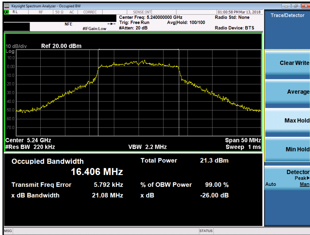
Plot 7-32. 26dB Bandwidth Plot (802.11a (UNII Band 1) – Ch. 48)
