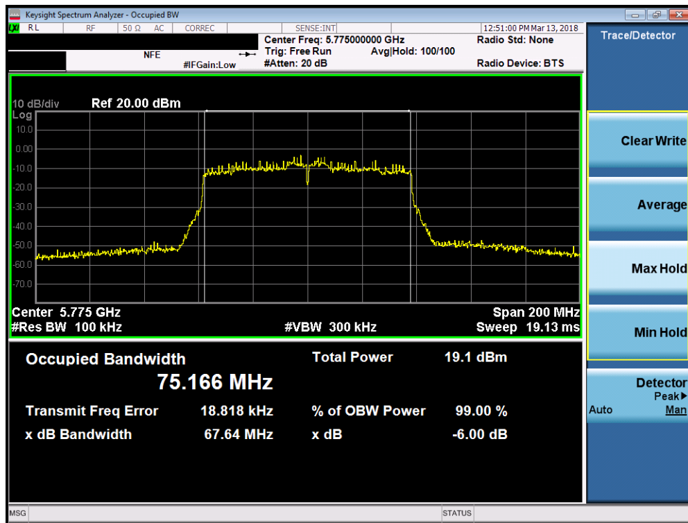
Plot 7-67. 6dB Bandwidth Plot (80MHz BW 802.11ac (UNII Band 3) – Ch. 155)
