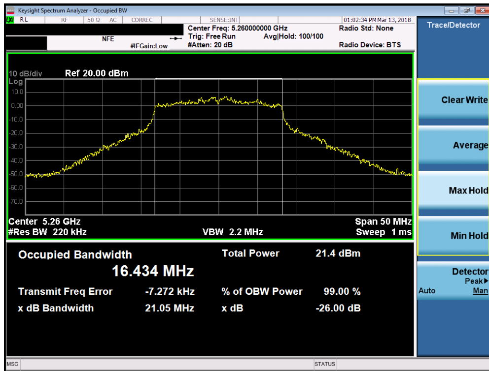
Plot 7-39. 26dB Bandwidth Plot (802.11a (UNII Band 2A) – Ch. 52)
