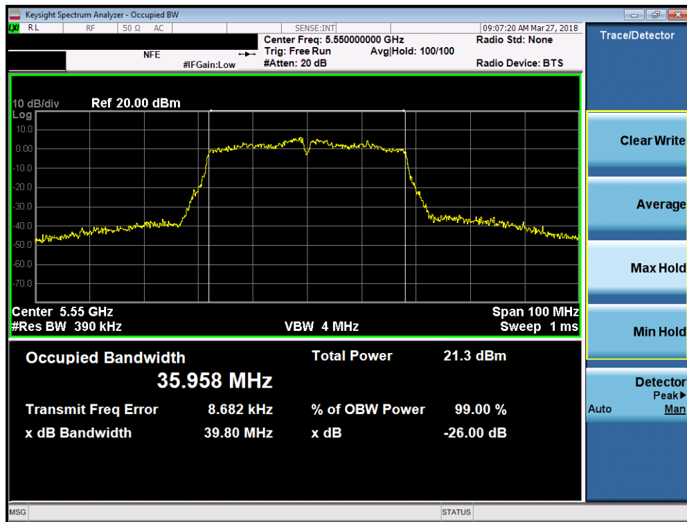
Plot 7-26. 26dB Bandwidth Plot (40MHz BW 802.11n (UNII Band 2C) – Ch. 110)
