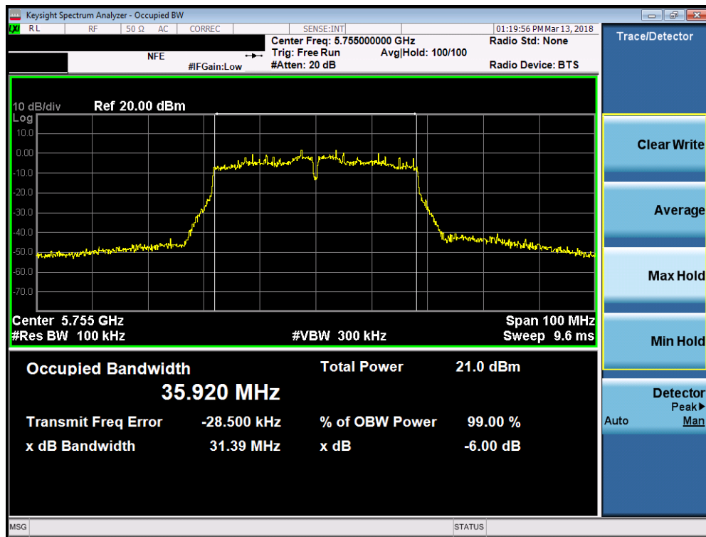
Plot 7-74. 6dB Bandwidth Plot (40MHz BW 802.11n (UNII Band 3) – Ch. 151)
