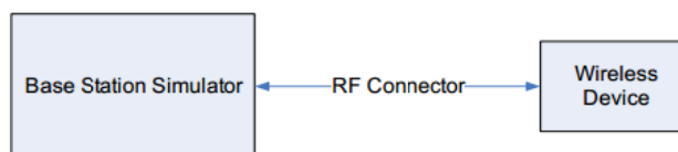
Figure 10.1 Power Measurement Setup
