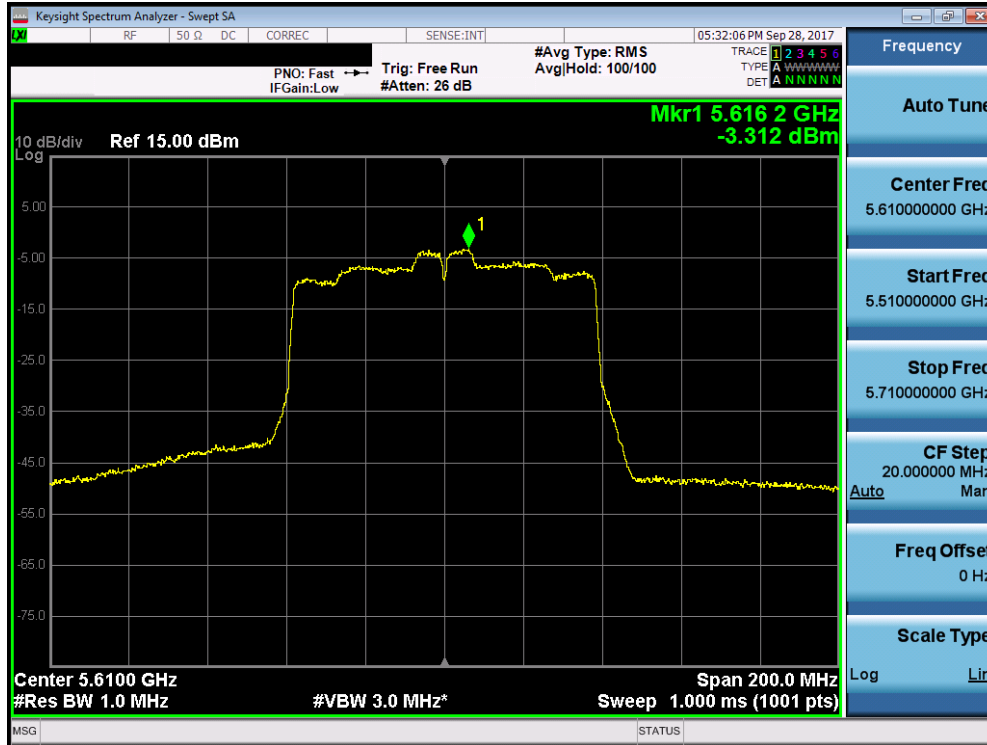
Plot 7-118. Power Spectral Density Plot (80MHz BW 802.11ac (UNII Band 2C) – Ch. 122)
