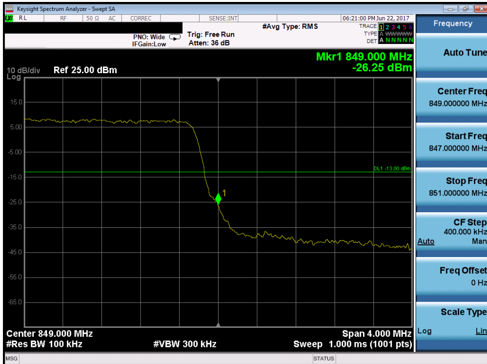
Plot 7-189. Upper Band Edge Plot (Band 5/26 – 5.0MHz QPSK – RB Size 25)
