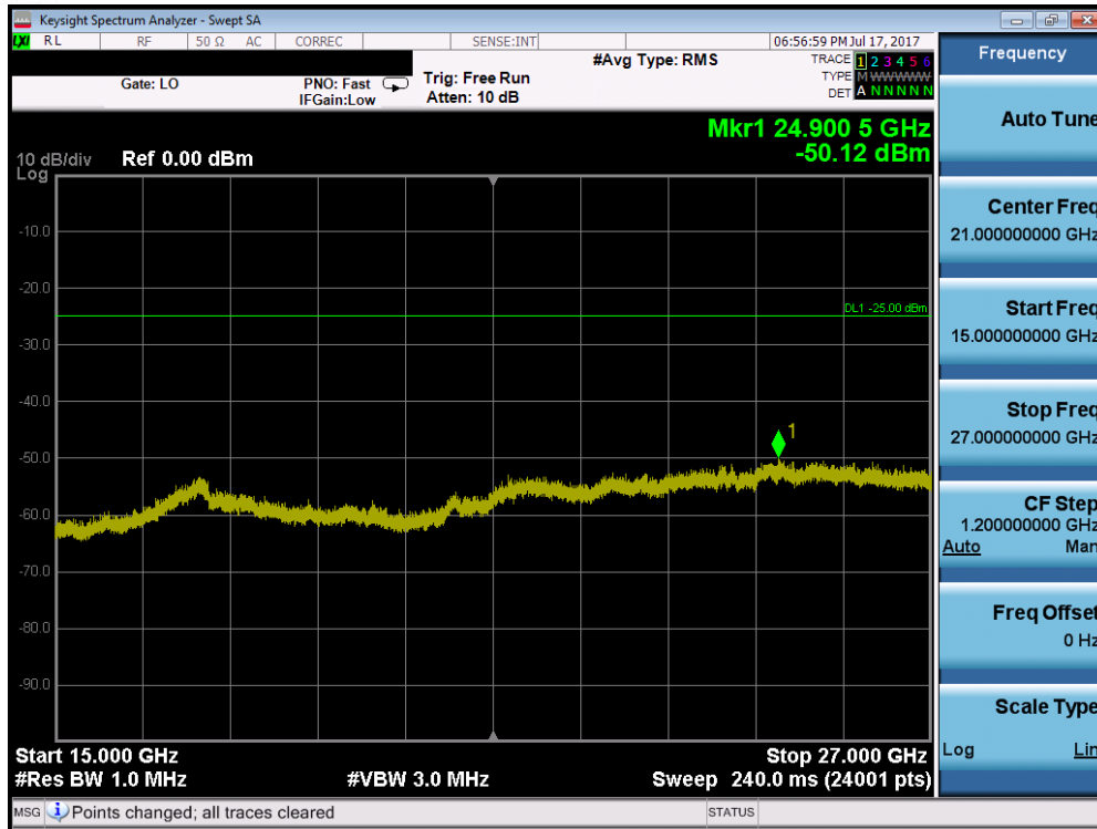
Plot 7-162. Conducted Spurious Plot (Band 41 – 15.0MHz QPSK – RB Size 1, RB Offset 0 – Mid Channel)
