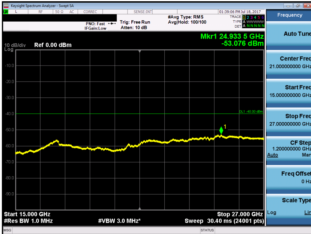
Plot 7-147. Conducted Spurious Plot (Band 30 – 10.0MHz QPSK – RB Size 1, RB Offset 0 – Mid Channel)
