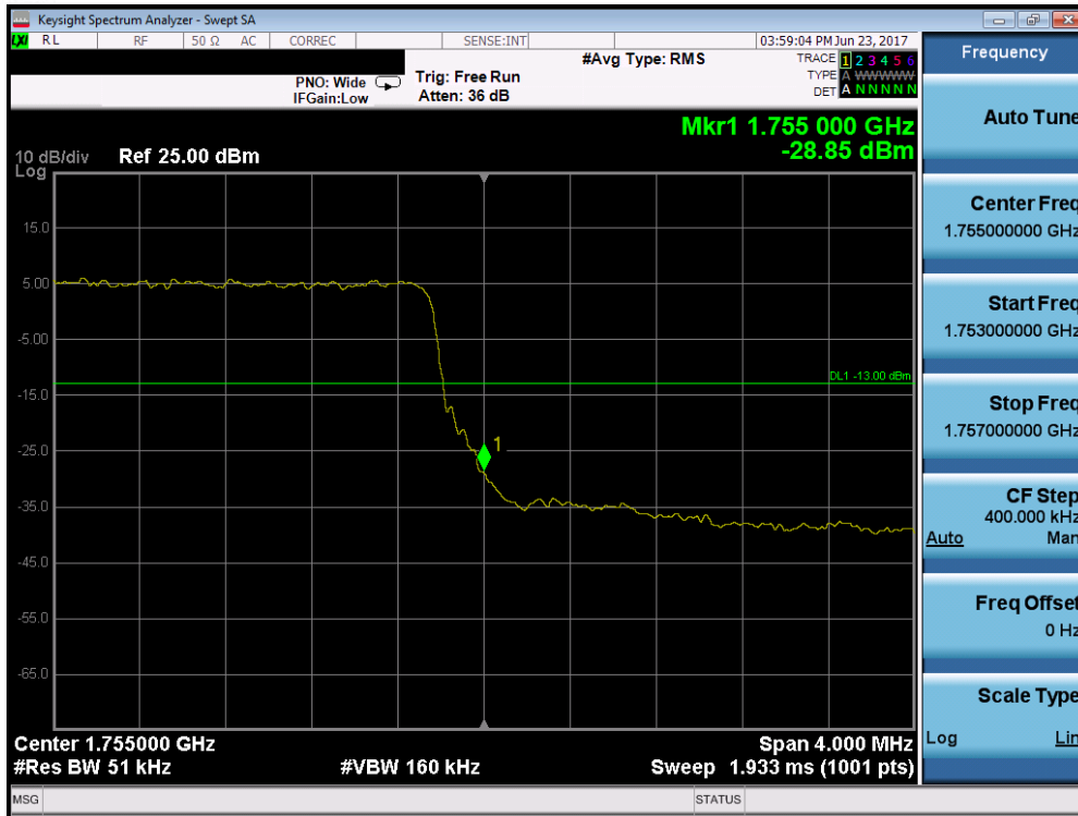
Plot 7-222. Upper Band Edge Plot (Band 4 – 5.0MHz QPSK – RB Size 25)
