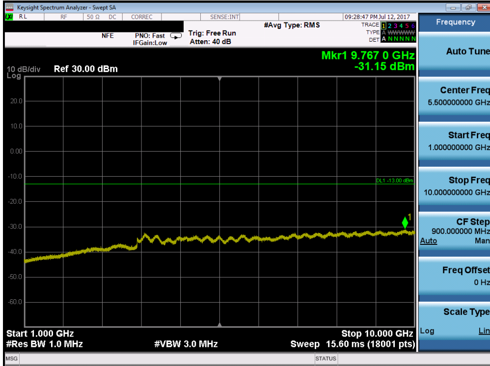
Plot 7-108. Conducted Spurious Plot (Band 12 – 3.0MHz QPSK – RB Size 1, RB Offset 0 – High Channel)
