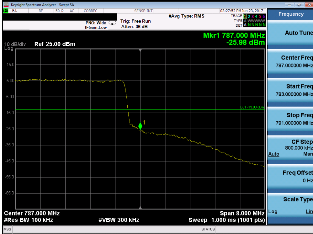
Plot 7-182. Upper Band Edge Plot (Band 13 – 10.0MHz QPSK – RB Size 50)
