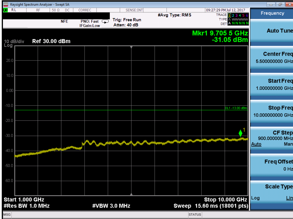
Plot 7-102. Conducted Spurious Plot (Band 12 – 3.0MHz QPSK – RB Size 1, RB Offset 0 – Low Channel)
