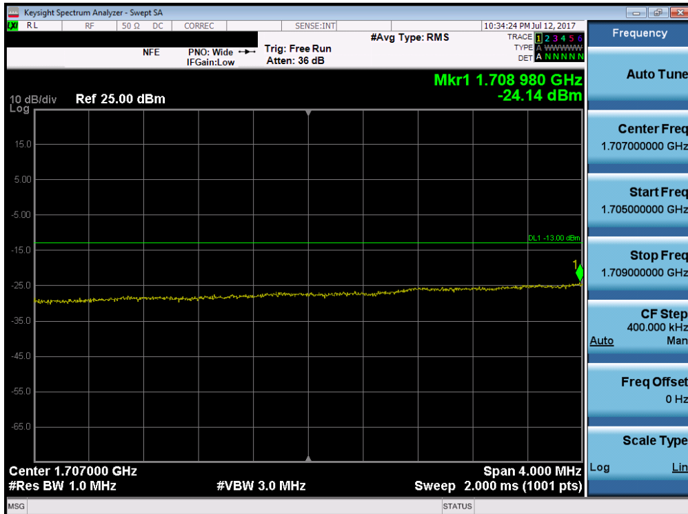
Plot 7-211. Lower Extended Band Edge Plot (Band 66/4 – 15.0MHz QPSK – RB Size 75)
