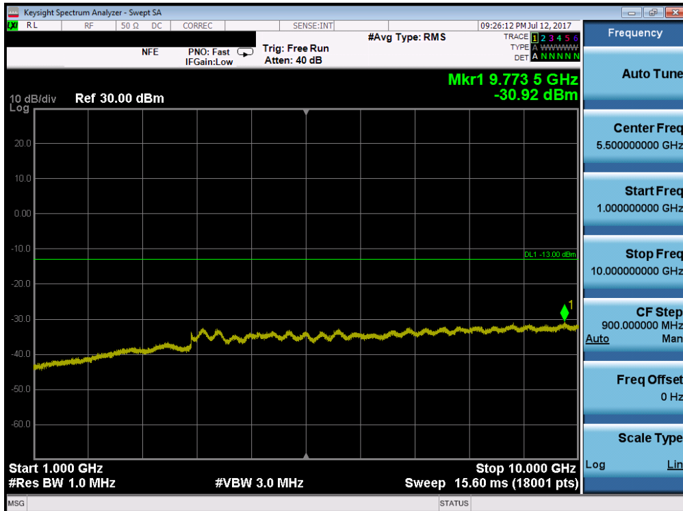
Plot 7-105. Conducted Spurious Plot (Band 12 – 3.0MHz QPSK – RB Size 1, RB Offset 0 – Mid Channel)
