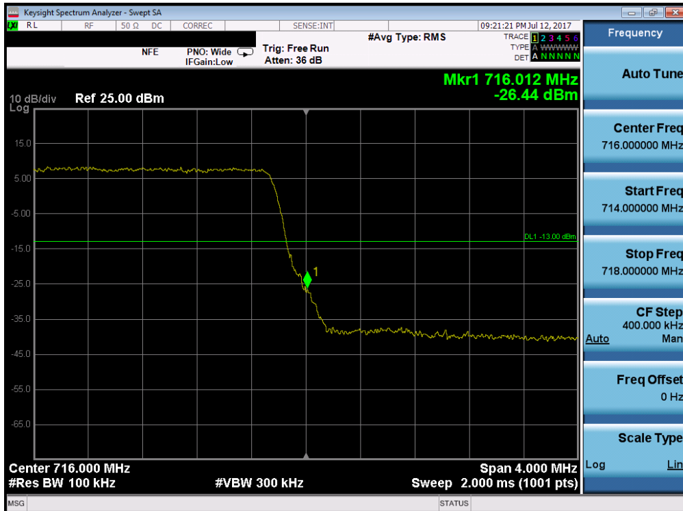
Plot 7-171. Upper Band Edge Plot (Band 12/17 – 5.0MHz QPSK – RB Size 25)
