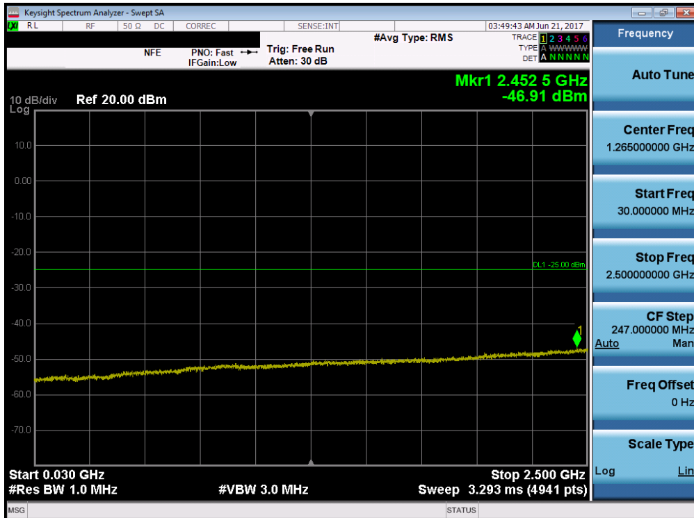
Plot 7-151. Conducted Spurious Plot (Band 7 – 20.0MHz QPSK – RB Size 1, RB Offset 0 – Mid Channel)
