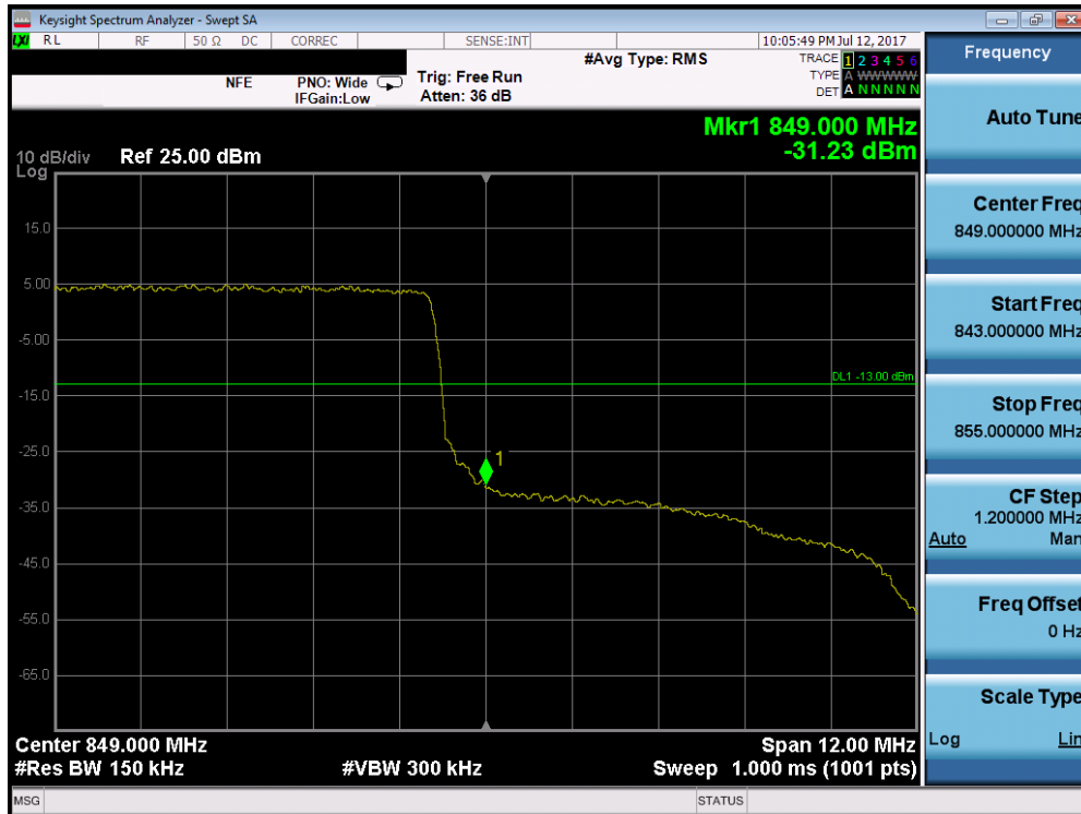
Plot 7-193. Upper Band Edge Plot (Band 26 – 15.0MHz QPSK – RB Size 75)
