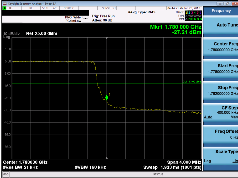
Plot 7-204. Upper Band Edge Plot (Band 66 – 5.0MHz QPSK – RB Size 25)
