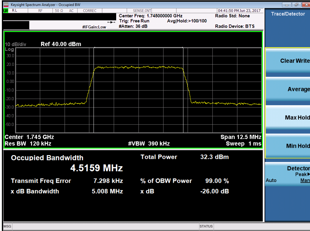
Plot 7-41. Occupied Bandwidth Plot (Band 4/66 – 5.0MHz 16-QAM – RB Size 25)
