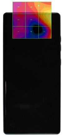
Figure 17-6 E-Field WD Scan overlay (T-Coil Centered scan area pictured)
