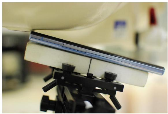
SAR Test Setup Photo 3 - Right Tilt
