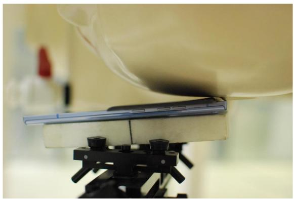
SAR Test Setup Photo 5 - Left Cheek with Mechanical Mode Position #3
