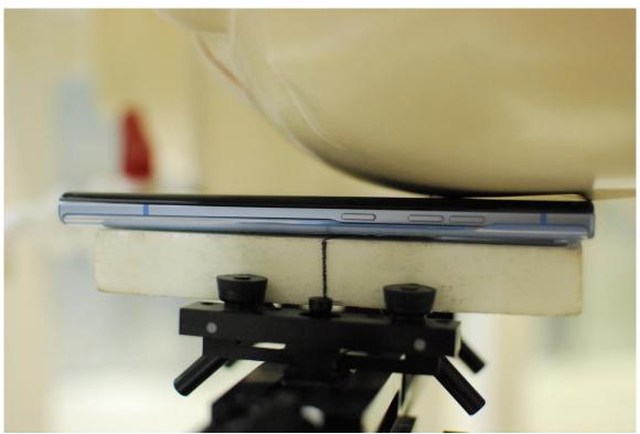
SAR Test Setup Photo 4 - Left Cheek
