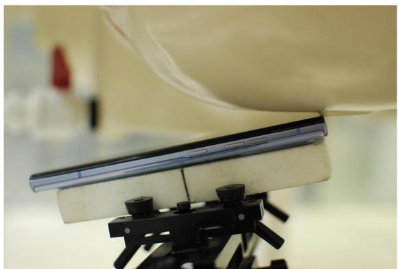
SAR Test Setup Photo 6 - Left Tilt
