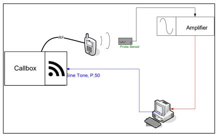
Figure 4-2 T-Coil Test Setup
