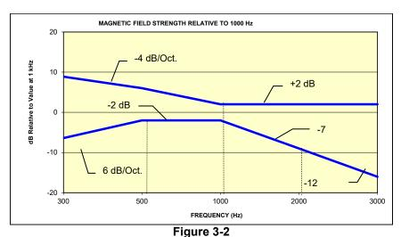
Magnetic Field frequency response for wireless devices with an axial field that exceeds -15 dB(A/m) at 1 kHz
