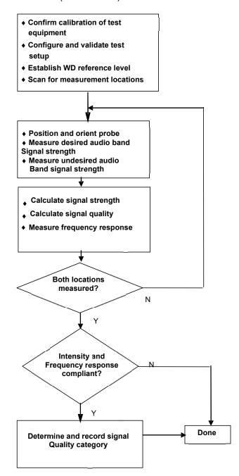
Figure 4-14 C63.19 T-Coil Signal Test Process
