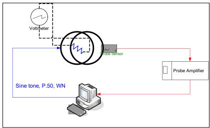
Figure 4-1 Validation Setup with Helmholtz Coil
