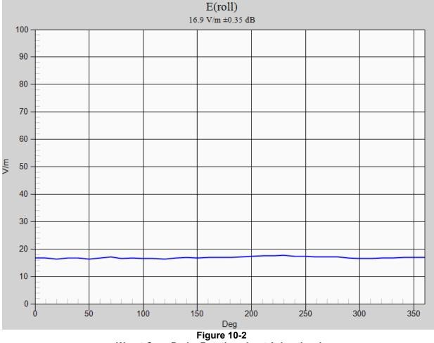
Worst-Case Probe Rotation about Azimuth axis
