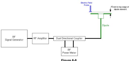
Figure 6-8 System Check Setup
