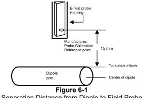
Separation Distance from Dipole to Field Probe
