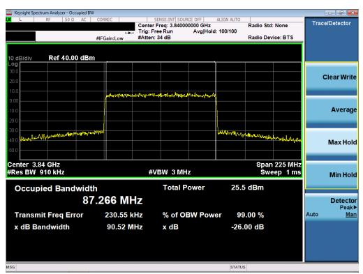
Plot 7-10. Occupied Bandwidth Plot (NR Band n77 - 90MHz 256-QAM - Full RB Configuration)
