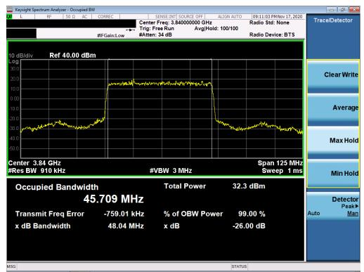
Plot 7-21. Occupied Bandwidth Plot (NR Band n77 - 50MHz π/2 BPSK - Full RB Configuration)
