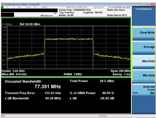
Plot 7-14. Occupied Bandwidth Plot (NR Band n77 - 80MHz 64-QAM - Full RB Configuration)
