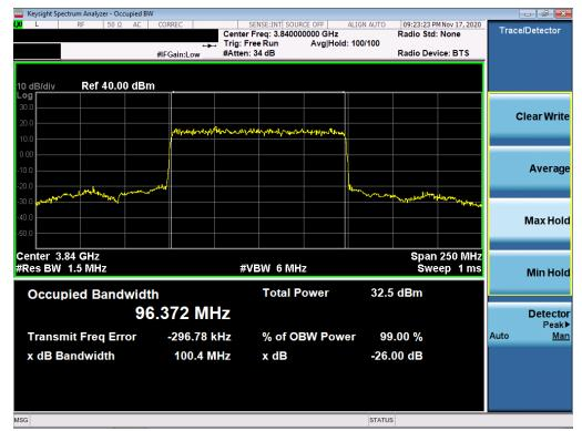
Plot 7-1. Occupied Bandwidth Plot (NR Band n77 - 100MHz π/2 BPSK - Full RB Configuration)
