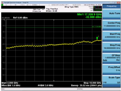
Plot 7-43. Conducted Spurious Plot (NR Band n77 - 100MHz QPSK - RB Size 1, RB Offset 0 - High Channel)
