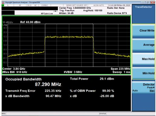
Plot 7-7. Occupied Bandwidth Plot (NR Band n77 - 90MHz QPSK - Full RB Configuration)
