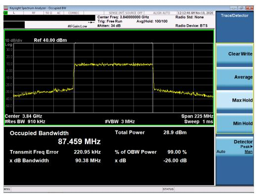
Plot 7-8. Occupied Bandwidth Plot (NR Band n77 - 90MHz 16-QAM - Full RB Configuration)
