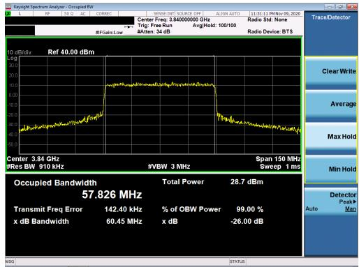
Plot 7-19. Occupied Bandwidth Plot (NR Band n77 - 60MHz 64-QAM - Full RB Configuration)
