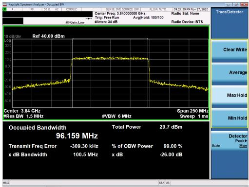
Plot 7-4. Occupied Bandwidth Plot (NR Band n77 - 100MHz 64-QAM - Full RB Configuration)
