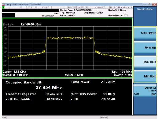
Plot 7-28. Occupied Bandwidth Plot (NR Band n77 - 40MHz 16-QAM - Full RB Configuration)
