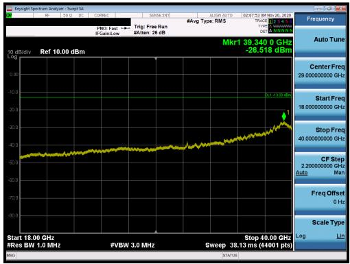
Plot 7-38. Conducted Spurious Plot (NR Band n77 - 100MHz QPSK - RB Size 1, RB Offset 0 - Low Channel)
