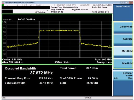
Plot 7-27. Occupied Bandwidth Plot (NR Band n77 - 40MHz QPSK - Full RB Configuration)
