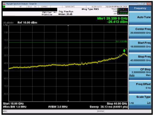
Plot 7-44. Conducted Spurious Plot (NR Band n77 - 100MHz QPSK - RB Size 1, RB Offset 0 - High Channel)
