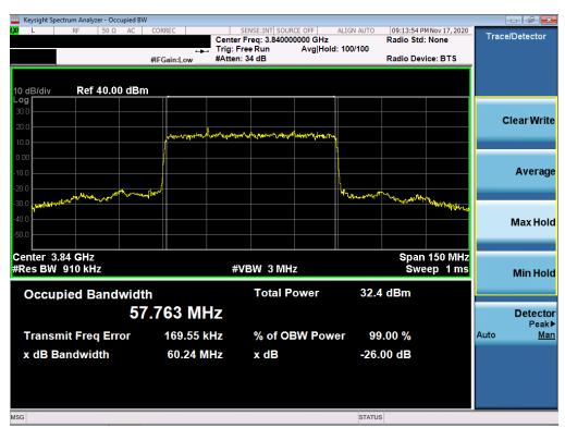
Plot 7-16. Occupied Bandwidth Plot (NR Band n77 - 60MHz π/2 BPSK - Full RB Configuration)
