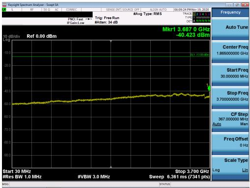
Plot 7-42. Conducted Spurious Plot (NR Band n77 - 100MHz QPSK - RB Size 1, RB Offset 0 - High Channel)
