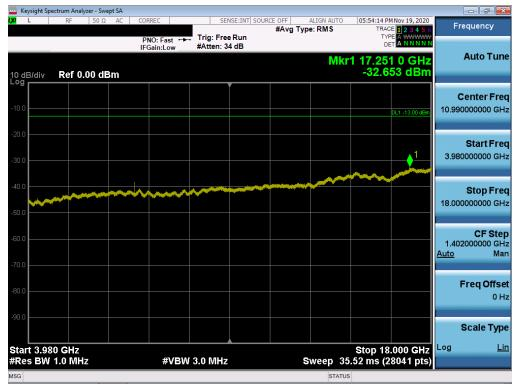
Plot 7-40. Conducted Spurious Plot (NR Band n77 - 100MHz QPSK - RB Size 1, RB Offset 0 - Mid Channel)
