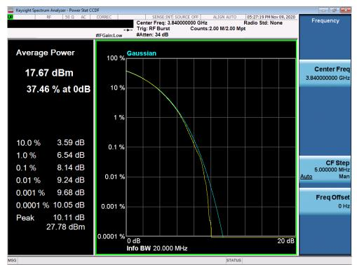
Plot 7-97. Peak to Average Ratio (NR Band n77 - 20MHz CP 256-QAM - Full RB Configuration)
