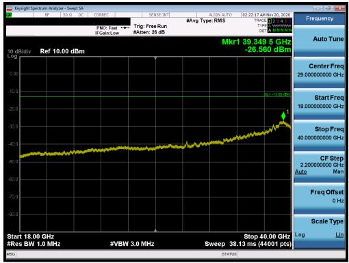
Plot 7-41. Conducted Spurious Plot (NR Band n77 - 100MHz QPSK - RB Size 1, RB Offset 0 - Mid Channel)
