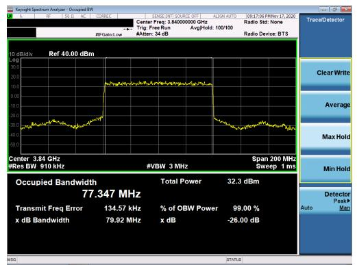
Plot 7-11. Occupied Bandwidth Plot (NR Band n77 - 80MHz π/2 BPSK - Full RB Configuration)
