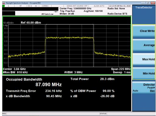
Plot 7-9. Occupied Bandwidth Plot (NR Band n77 - 90MHz 64-QAM - Full RB Configuration)
