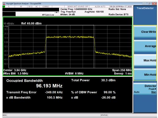
Plot 7-3. Occupied Bandwidth Plot (NR Band n77 - 100MHz 16-QAM - Full RB Configuration)
