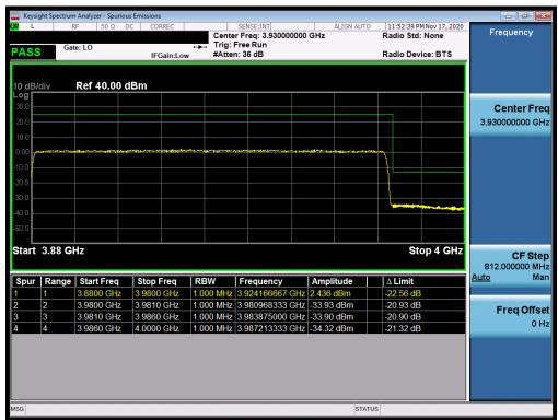
Plot 7-46. Upper Band Edge Plot (NR Band n77 - 100MHz CP-OFDM-QPSK - Full RB Configuration)
