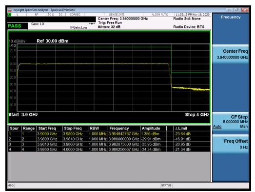
Plot 7-50. Upper Band Edge Plot (NR Band n77 - 80MHz CP-OFDM-QPSK - Full RB Configuration)
