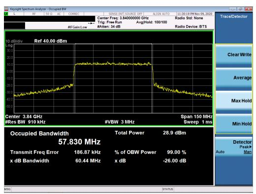
Plot 7-18. Occupied Bandwidth Plot (NR Band n77 - 60MHz 16-QAM - Full RB Configuration)
