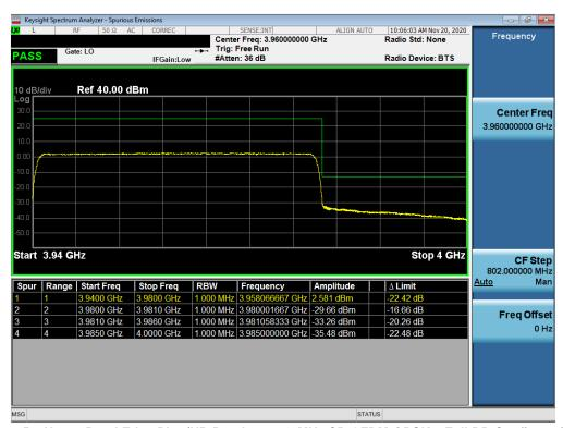
Plot 7-56. Upper Band Edge Plot (NR Band n77 - 40MHz CP-OFDM-QPSK - Full RB Configuration)
