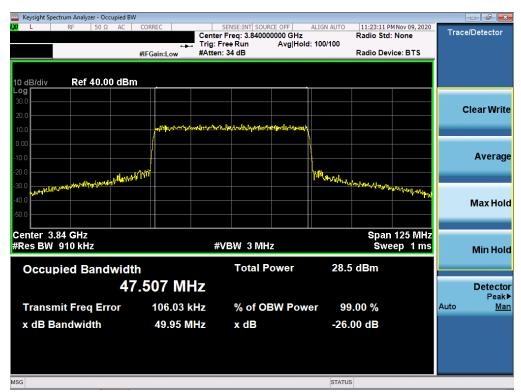
Plot 7-24. Occupied Bandwidth Plot (NR Band n77 - 50MHz 64-QAM - Full RB Configuration)
