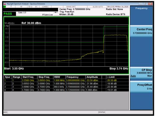
Plot 7-55. Lower Band Edge Plot (NR Band n77 - 40MHz CP-OFDM-QPSK - Full RB Configuration)
