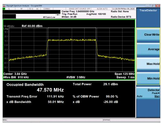
Plot 7-22. Occupied Bandwidth Plot (NR Band n77 - 50MHz QPSK - Full RB Configuration)
