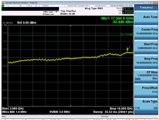
Plot 7-37. Conducted Spurious Plot (NR Band n77 - 100MHz QPSK - RB Size 1, RB Offset 0 - Low Channel)
