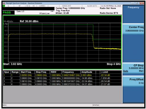
Plot 7-52. Upper Band Edge Plot (NR Band n77 - 60MHz CP-OFDM-QPSK - Full RB Configuration)
