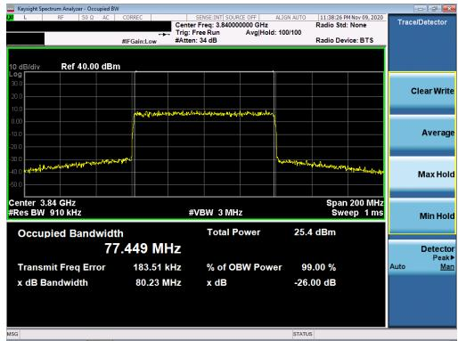
Plot 7-15. Occupied Bandwidth Plot (NR Band n77 - 80MHz 256-QAM - Full RB Configuration)
