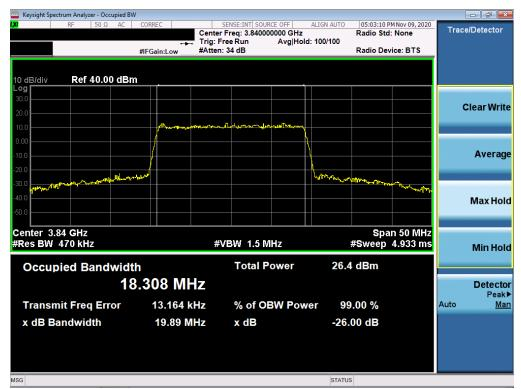
Plot 7-35. Occupied Bandwidth Plot (NR Band n77 - 20MHz 256-QAM - Full RB Configuration)
