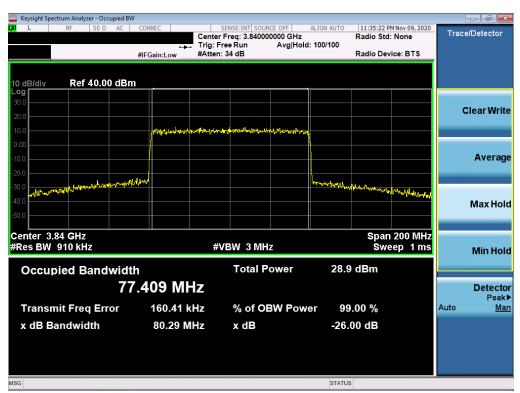
Plot 7-12. Occupied Bandwidth Plot (NR Band n77 - 80MHz QPSK - Full RB Configuration)
