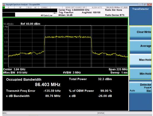
Plot 7-6. Occupied Bandwidth Plot (NR Band n77 - 90MHz π/2 BPSK - Full RB Configuration)
