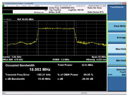
Plot 7-31. Occupied Bandwidth Plot (NR Band n77 - 20MHz π/2 BPSK - Full RB Configuration)
