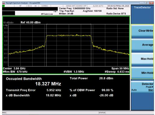
Plot 7-33. Occupied Bandwidth Plot (NR Band n77 - 20MHz 16-QAM - Full RB Configuration)
