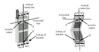
Figure 5-3 Handset Vertical Center & Horizontal Line Reference Points
