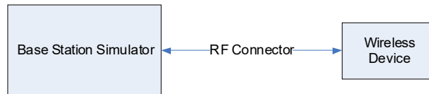
Figure 9-2 Power Measurement Setup
