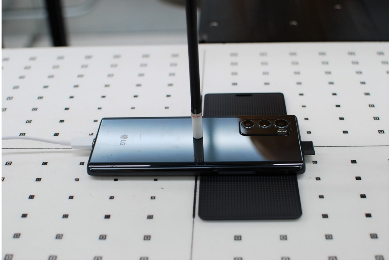
Figure D-9 Near Field Power Density Test Setup Photo – Back in Mechanical Mode #4 at 2mm
