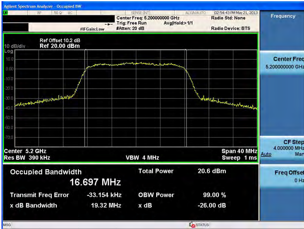
26 dB Bandwidth plot (802.11a-CH 40)
