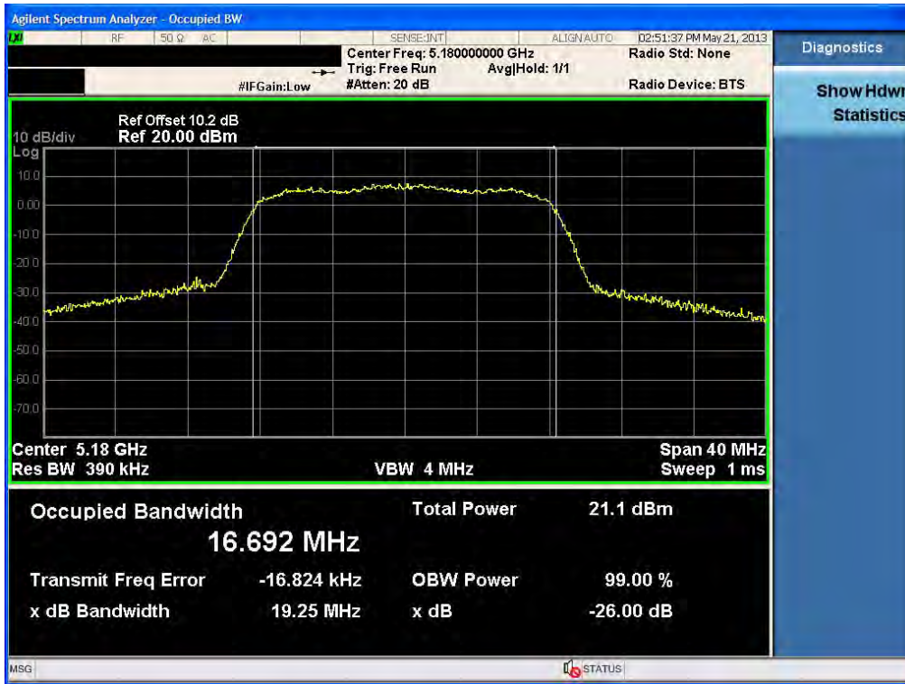
26 dB Bandwidth plot (802.11a-CH 40)
