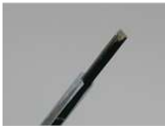
Figure 4.3 EX3DV4 E-field Probe
