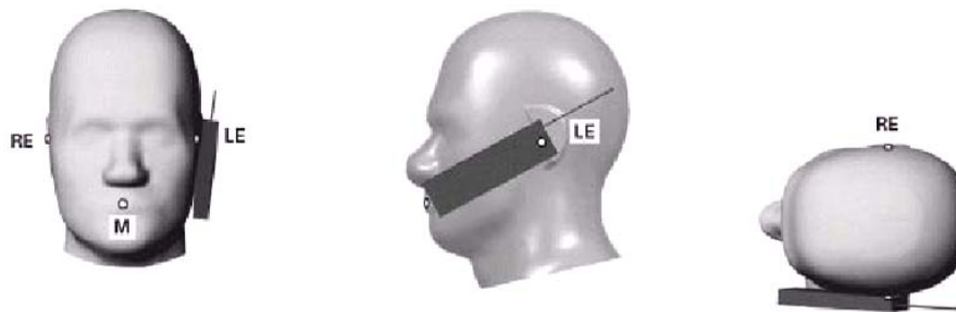
Figure 6.4 Front, Side and Top View of Cheek/Touch Position
