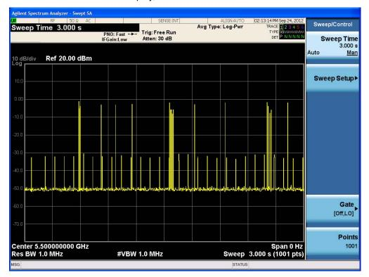
Time Display, WLAN Channel Traffic (Streaming Video)
