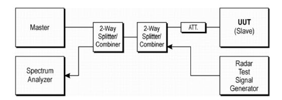
Figure 3-1. Conducted Test Setup for DFS
