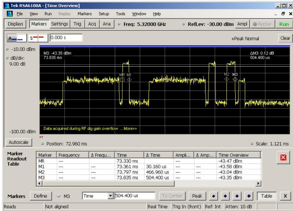
Figure 5-7. Pulse Width After 200ms
