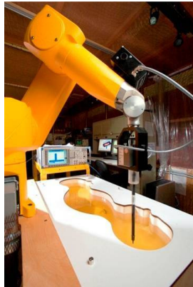
Figure 4-1 SAR Measurement System
