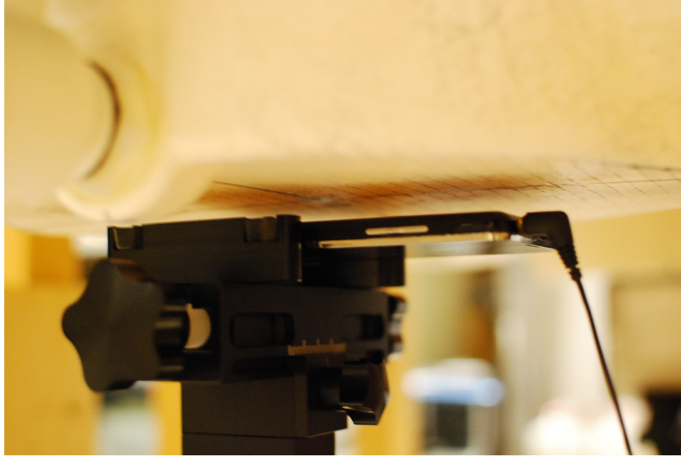
SAR Test Setup Photo 11: Body-Worn at 1.0 cm
