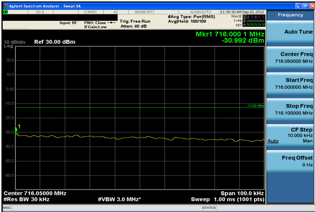
Plot 7-12. Upper Band Edge Plot (QPSK – RB Size 25)
