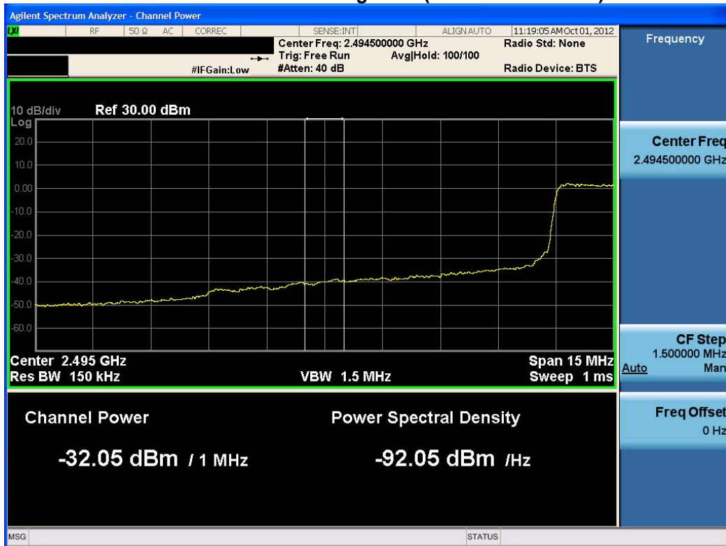
Plot 7-64. Lower Band Edge Plot (QPSK – RB Size 50)
