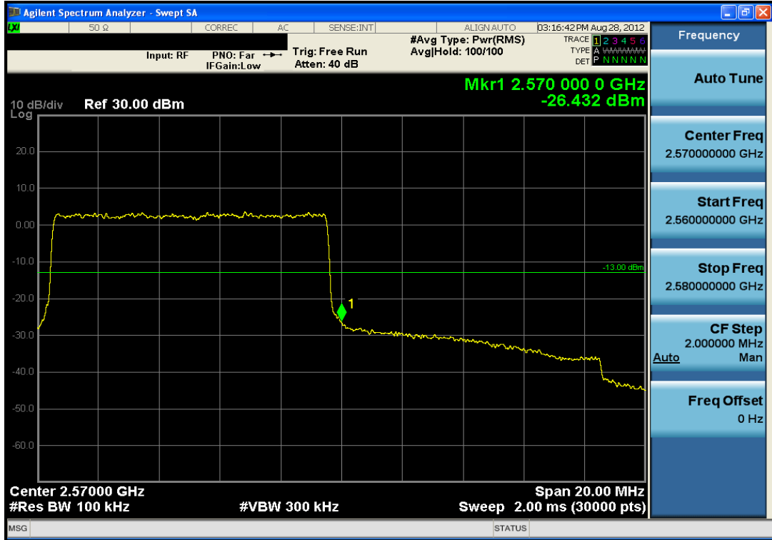
Plot 7-75. Upper Band Edge Plot (QPSK – RB Size 1, Offset 49)
