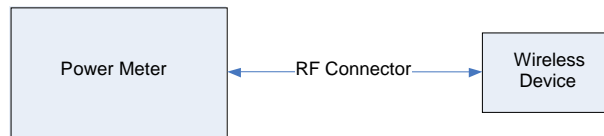
Figure 10-4 Power Measurement Setup
