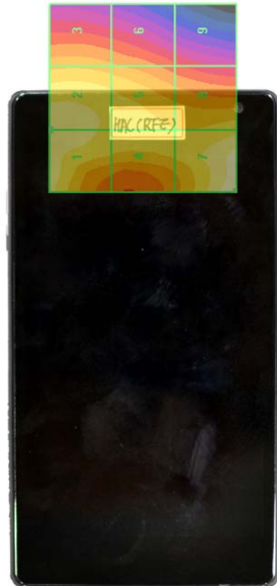
Figure 17-5 H-Field WD Scan overlay
