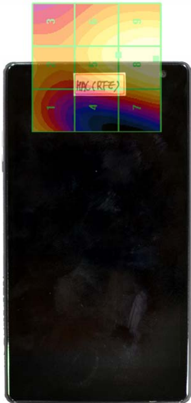
Figure 17-4 E-Field WD Scan overlay
