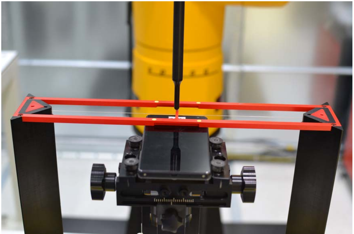
Figure 17-1 Ear Reference Point HAC Phantom Alignment
