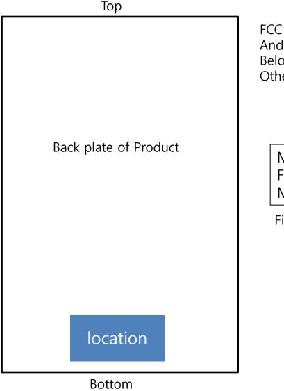
FCC ID is etched, near the bottom of the EUT. And customer do not remove this back cover. Below Fig.1 is representation of FCC Label information, Other informations may be include on the label.
