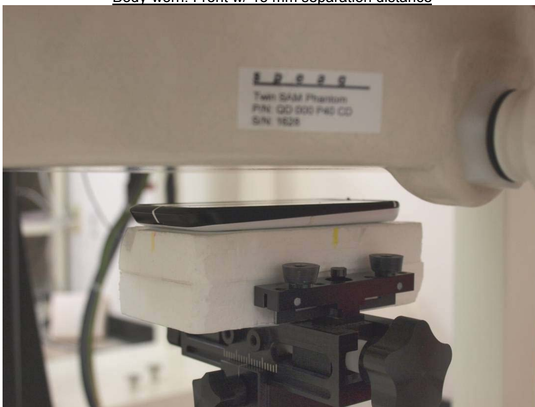
Body-worn: Front w/ 15 mm separation distance
