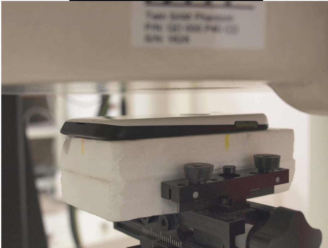
Body-worn: Rear w/ 15 mm separation distance
