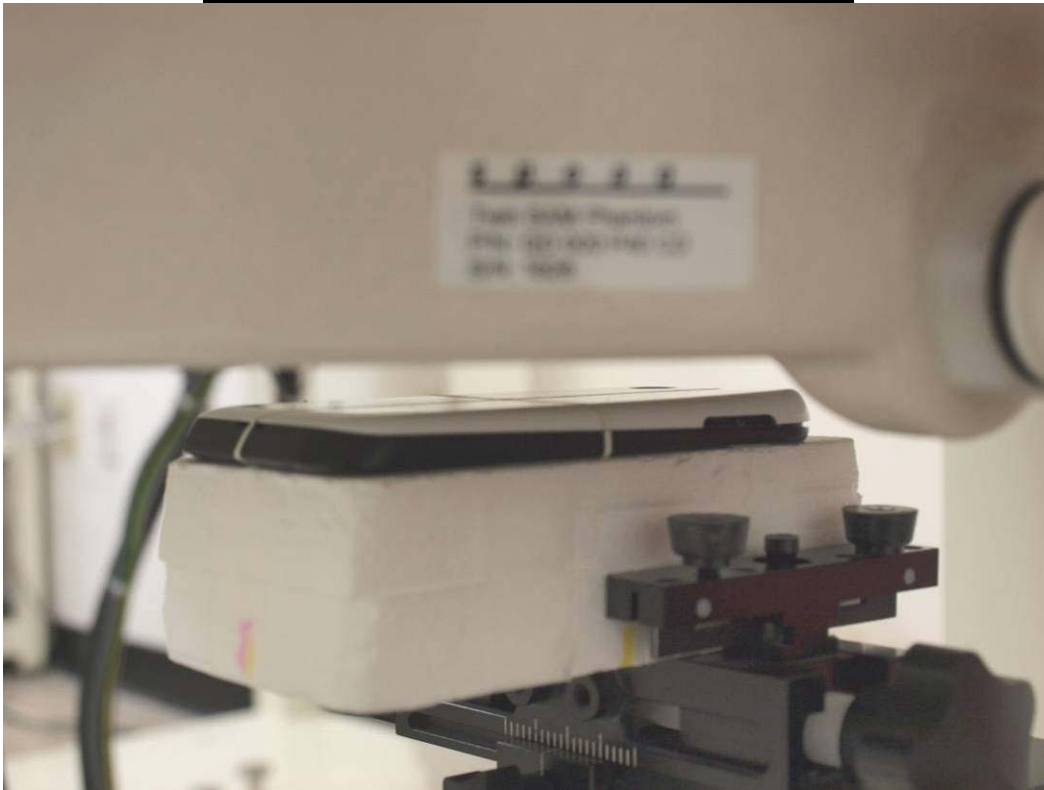
Body-hotspot: Rear w/ 10 mm separation distance with Headset (for WCDMA mode only)
