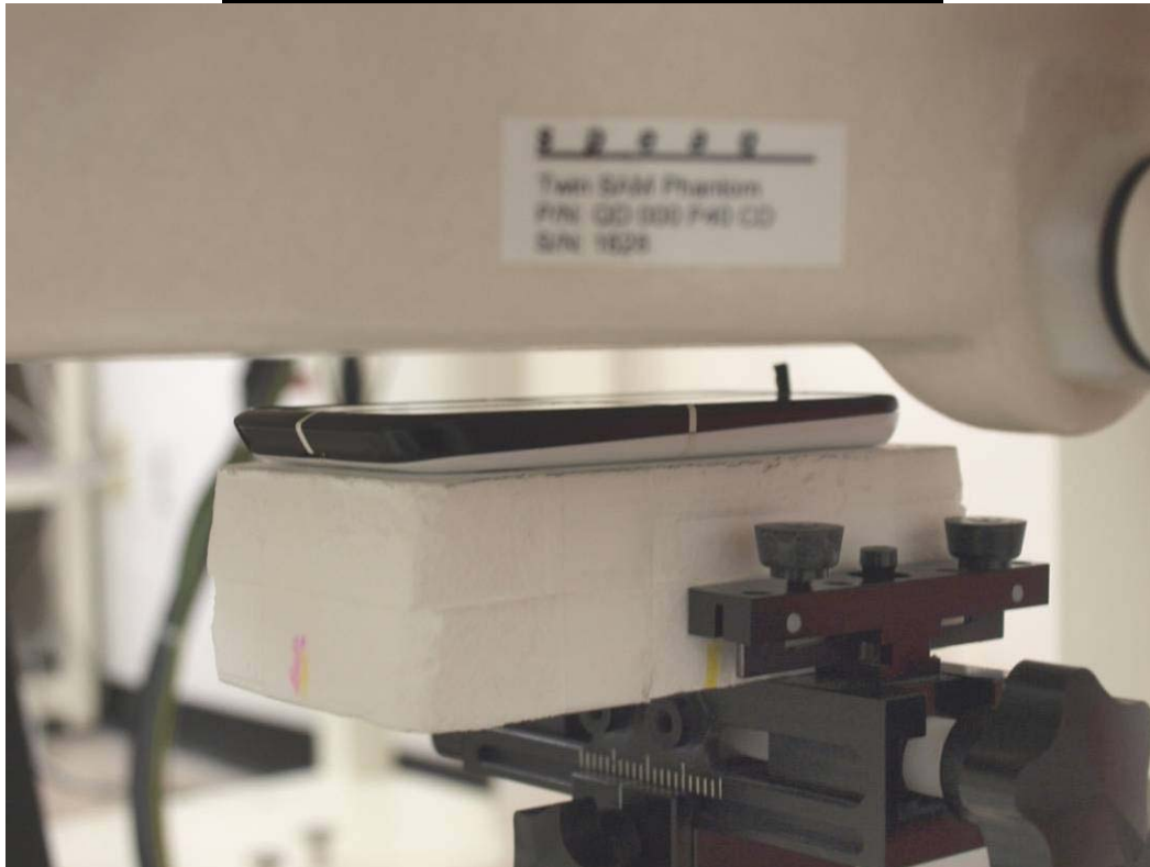
Body-hotspot: Front w/ 10 mm separation distance
