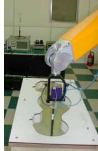
Figure 3.2 Photograph of the probe and the Phantom
