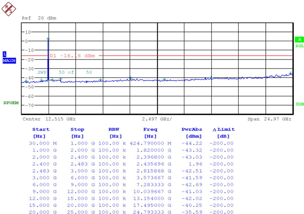
**High Band-edge** **Highest Channel** & Modulation: **802.11n (HT20)**
