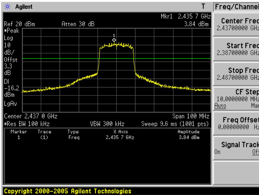
**Conducted Spurious Emissions** Middle Channel & Modulation: 802.11n (HT20)
