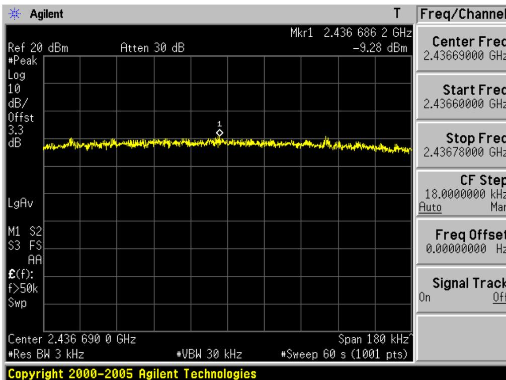
**Power Spectral Density**      **Highest Channel**    & Modulation: **802.11n (HT20)**
