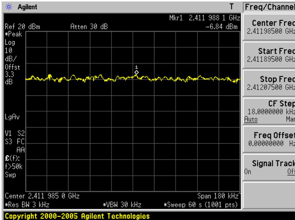
**Power Spectral Density**      **Middle Channel** & Modulation: **802.11b**
