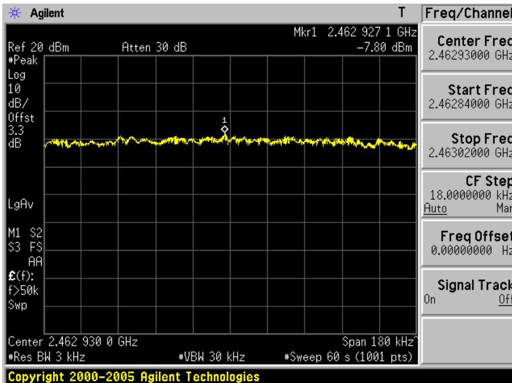
**Power Spectral Density**      **Lowest Channel** & Modulation: **802.11n (HT20)**
