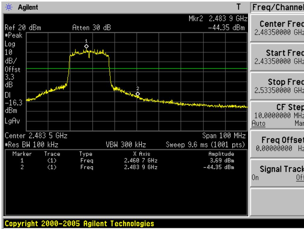
**Conducted Spurious Emissions** **Highest Channel** & Modulation: **802.11n (HT20)**
