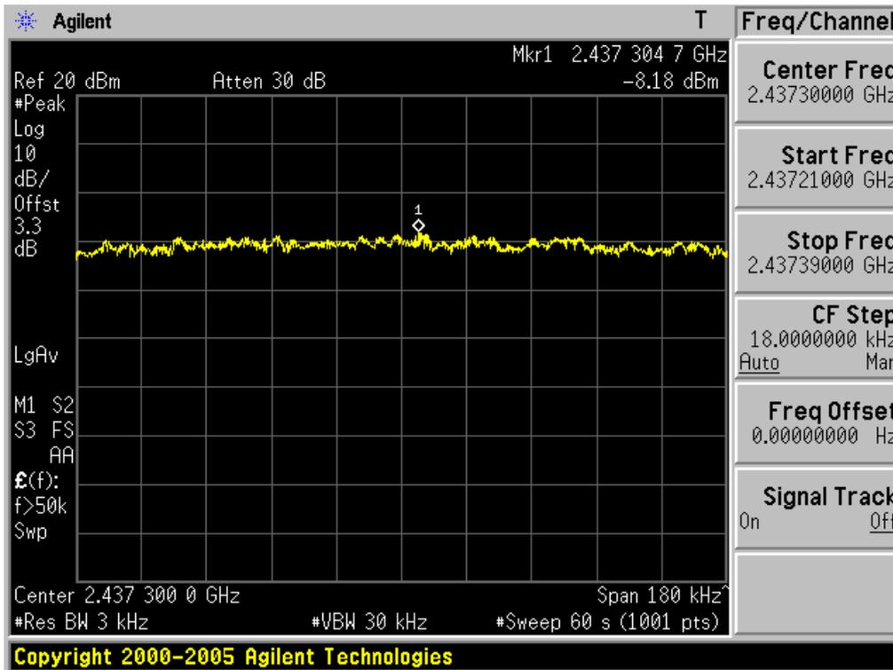
**Power Spectral Density**      **Highest Channel**    &    Modulation: **802.11g**
