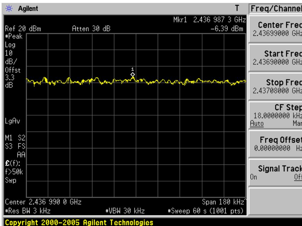
**Power Spectral Density**      **Highest Channel**    & Modulation: **802.11b**
