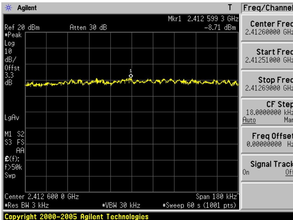
**Power Spectral Density**      **Middle Channel**    &    Modulation: **802.11g**
