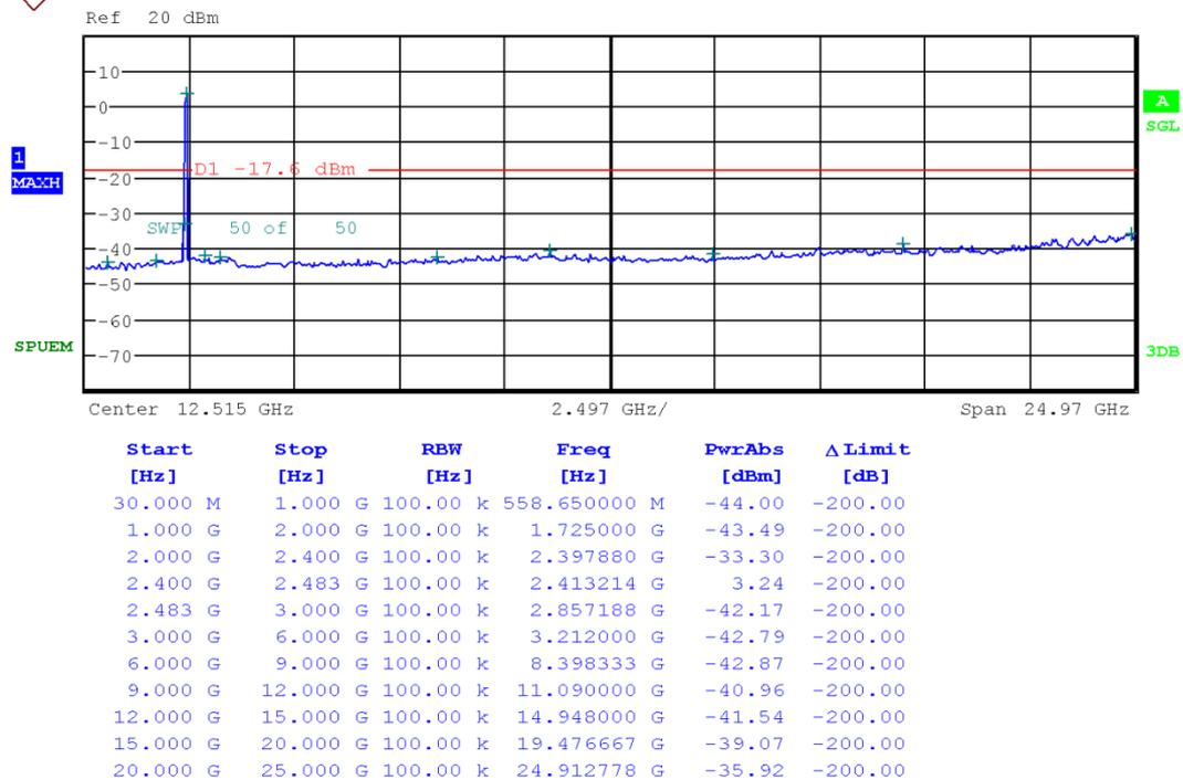
**Reference for limit** Middle Channel & Modulation: **802.11g**
