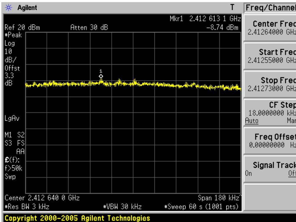
**Power Spectral Density**      **Middle Channel** & Modulation: **802.11n (HT20)**
