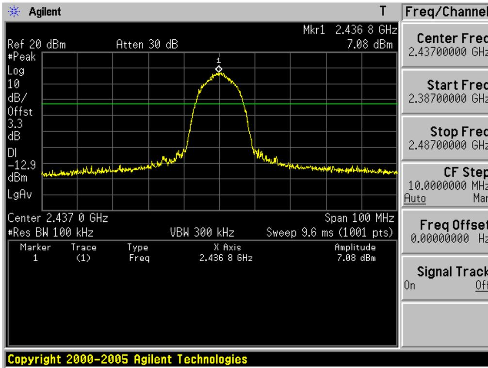
Conducted Spurious Emissions **Middle Channel** & Modulation: **802.11b**
