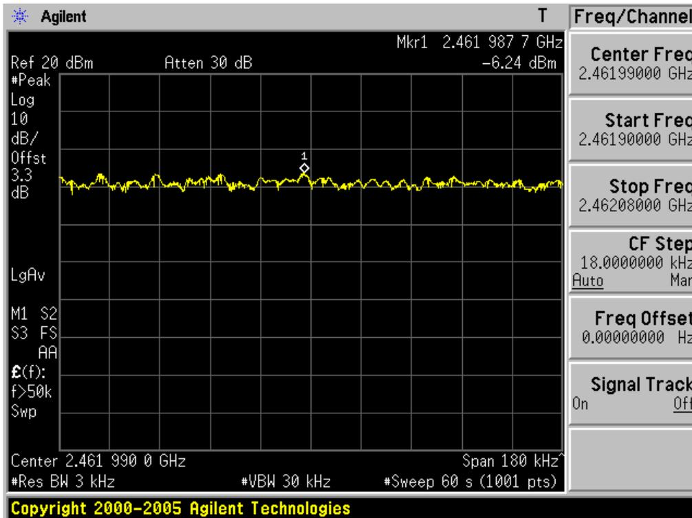
**Power Spectral Density**      **Lowest Channel**    & Modulation: **802.11g**
