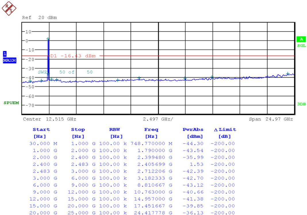
**Reference for limit** Middle Channel & Modulation: 802.11n (HT20)
