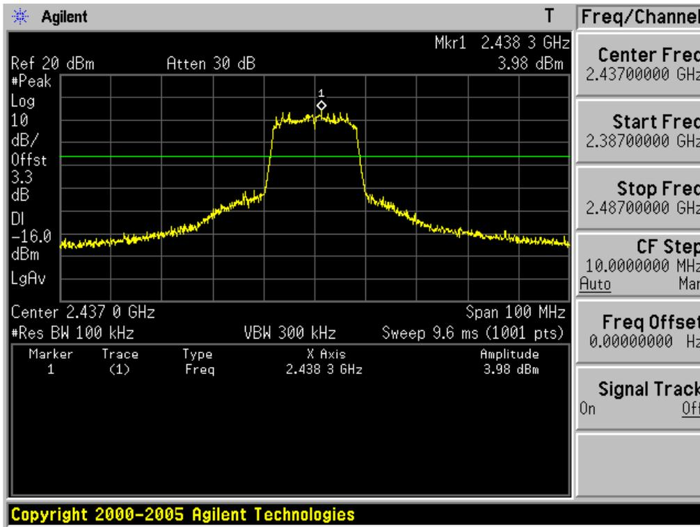
**Conducted Spurious Emissions** Middle Channel & Modulation: **802.11g**
