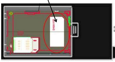
The label is located back of the phone. When the user install the battery, the user can see the label.
