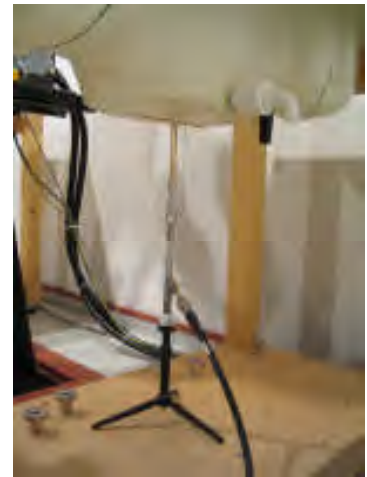
Photo of the dipole Antenna
