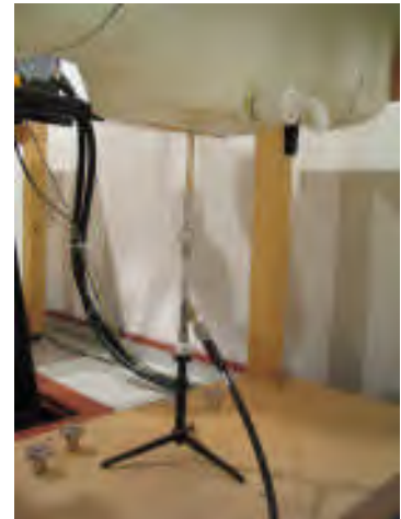
Photo of the dipole Antenna
