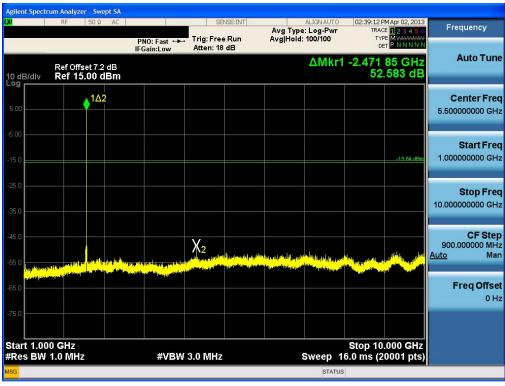
Test Plots ( $\pi$ /4DQPSK) - 1 GHz - 10 GHz (RBW:1 MHz, VBW: 1 MHz) Spurious Emission (Mid-CH)
