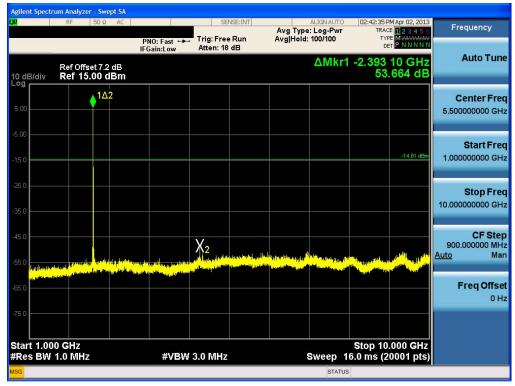
Test Plots (8DPSK) - 1 GHz - 10 GHz (RBW:1 MHz, VBW: 1 MHz) Spurious Emission (High-CH)
