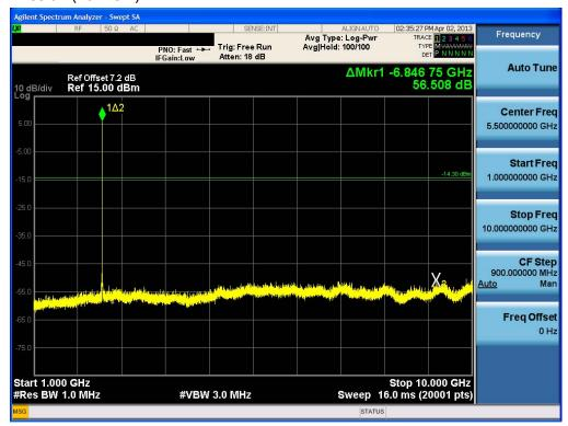
Test Plots (GFSK) - 1 GHz - 10 GHz (RBW:1 MHz, VBW: 1 MHz) Spurious Emission (Mid-CH)
