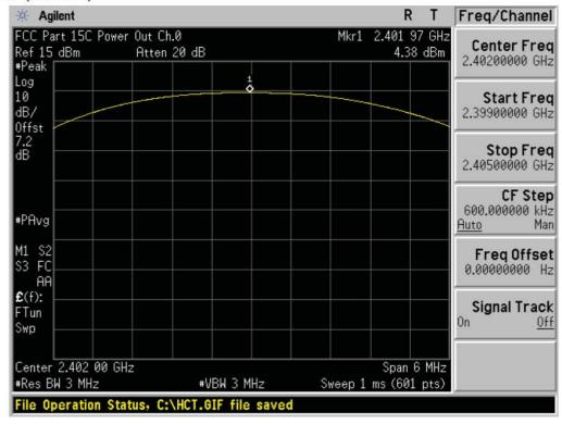
Test Plots (GFSK) Peak Power (Mid-CH)
