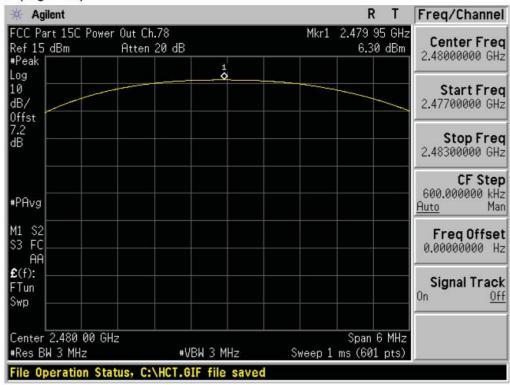
Test Plots (8DPSK) Peak Power (Low-CH)
