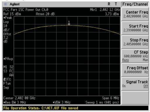
Test Plots (π/4DQPSK) Peak Power (Mid-CH)
