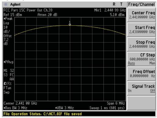
Test Plots (8DPSK) Peak Power (High-CH)
