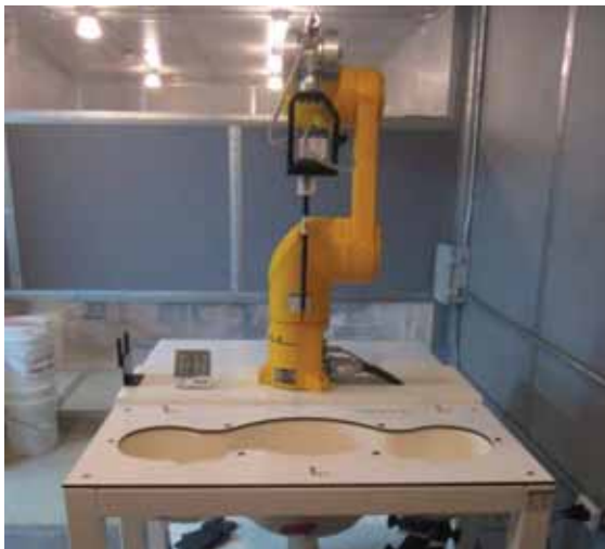
Figure 2.2 DASY5 Test System
