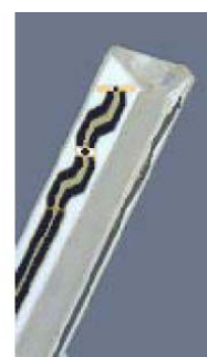
Figure 3.3 Probe Thick-Film Technique
