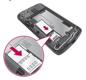
3 Insert the battery into place by aligning the gold contacts on the phone and the battery (1) and pressing it down until it clicks into place (2).
