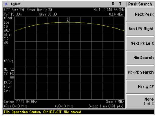
Test Plots (8DPSK) Peak Power (High-CH)
