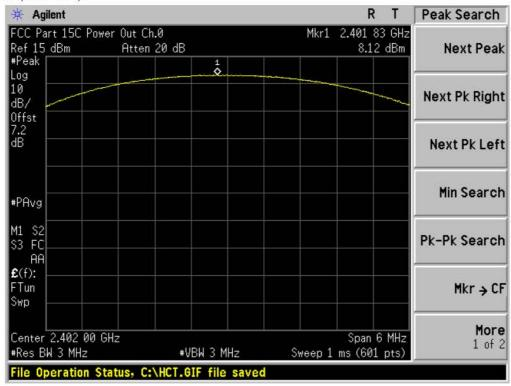
Test Plots (π/4DQPSK) Peak Power (Mid-CH)
