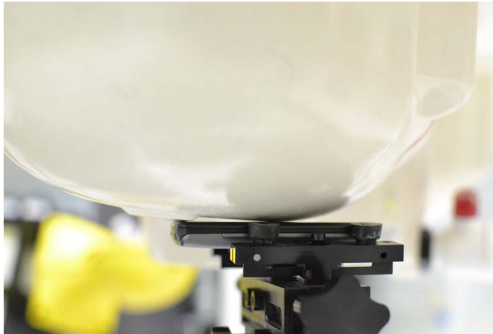
SAR Test Setup Photo 1 – Right Cheek
