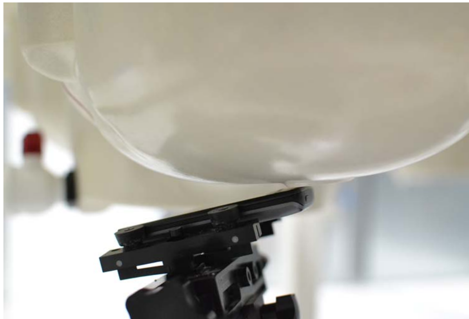
SAR Test Setup Photo 4 – Left Tilt
