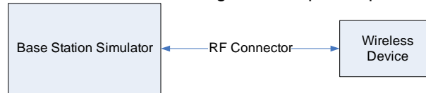
Figure 8-2 Power Measurement Setup
