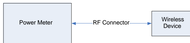
Figure 8-3 Power Measurement Setup
